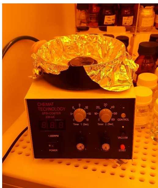
Figure 4.1 Chemat Scientific KW-4A Spin coater. When in use, the bowl is covered by a metal lid to prevent the resist from escaping.
