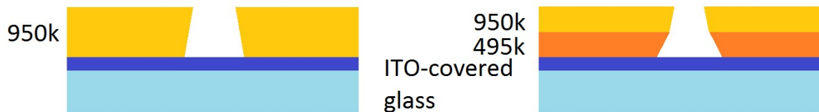
Figure 3.2 Illustration of resist schemes. The left figure shows a single layer resist, while the right shows a bi-layer resist.
