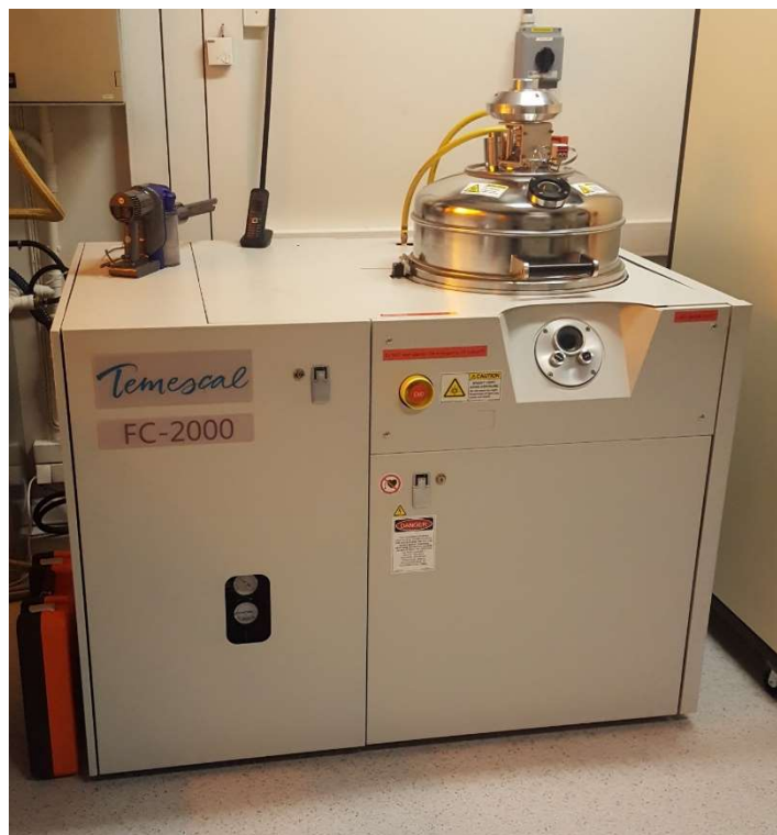
Figure 3.4 The Temescal FC-2000 electron beam evaporator. The sample is inserted into the process chamber via the dome on top of the machine.
