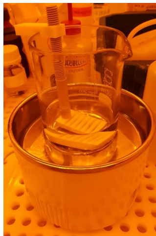
Figure 4.7 The sonicator setup. The sample holder could contain up to 6 coverslips at once.
