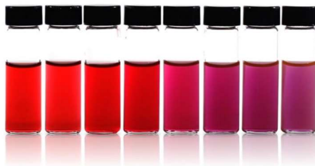
Figure 1.1 Gold nanoparticles of sizes 5-100 nm. The particles selectively absorb light based on the particle size, which is why golden particles with diameters below 100 nm appears red rather than the gold colour we are used to from the bulk material. Picture taken from the nanoComposix website, a nanoparticle manufacturer [7].
