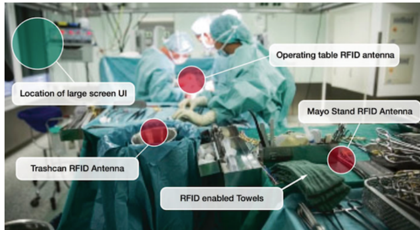
Figure 2.4: Locations of User interface(UI) and RFID antennas[4].
