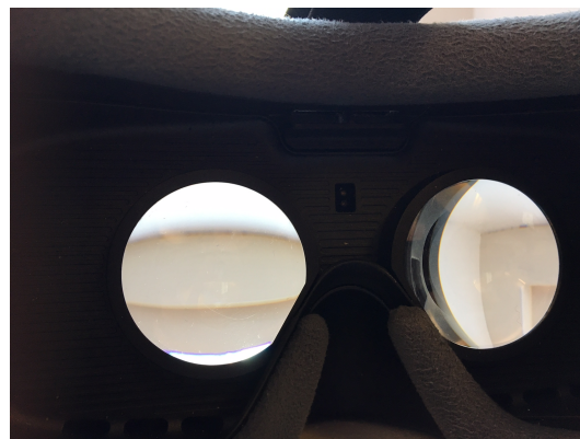
Figure 4.3: GEAR VR lenses and proximity sensor
