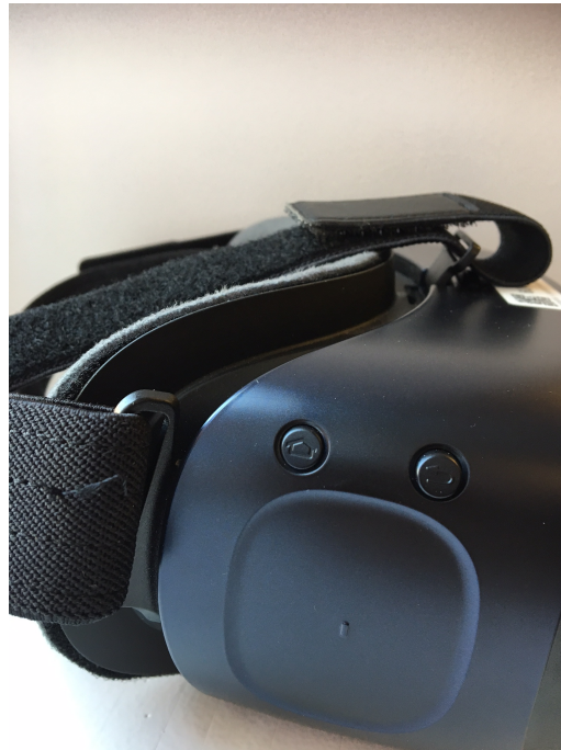
Figure 4.2: GEAR VR Touchpad and buttons
