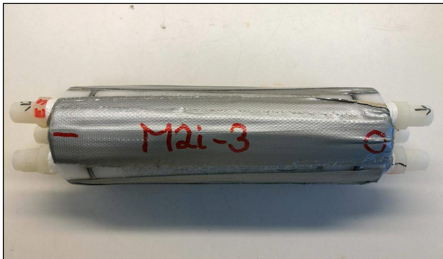
Figure 27 – Fractured marble core with duct tape holding the core pieces and end pieces together at sufficiently high pressure for foam generation.
