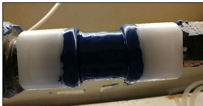
Figure 32 – Foam generator used during dynamic MRI of foam injection in core M2i-1.
