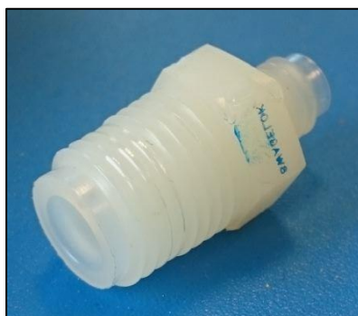
Figure A3 – Swagelok fittings were connected to each hole in the end pieces.
