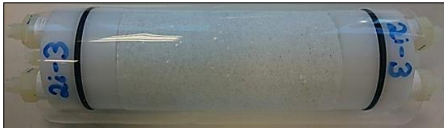
Figure 18 – Fractured marble core M2i-3 with end pieces, Swagelok fittings and shrink sleeve, before shrinking.
