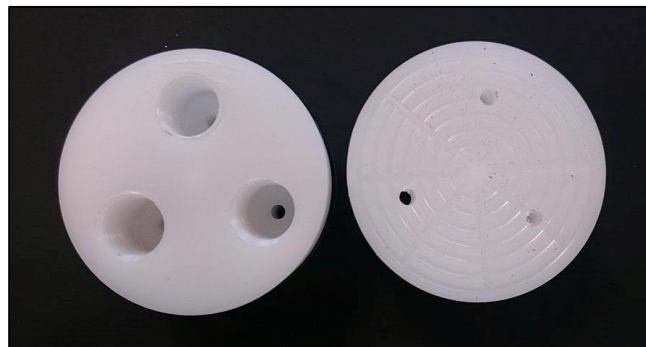
Figure 16 – End pieces designed for fractured marble cores.
