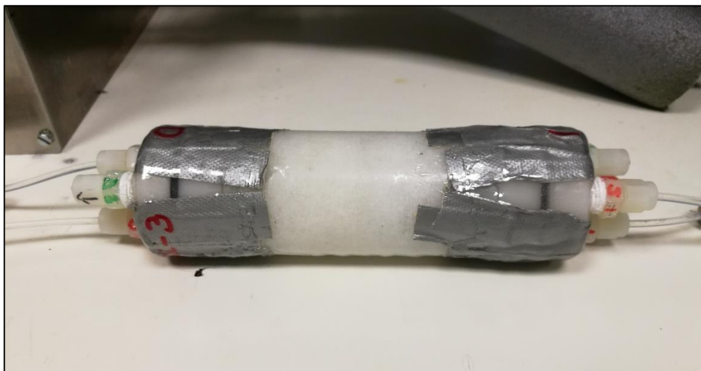
Figure 28 – Fractured marble core M2i-3 with two layers of epoxy, separated with duct tape, to hold end pieces and core pieces together during foam injection at 2 bar.
