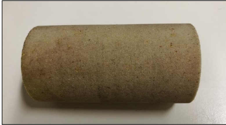
Figure 19 – A Bentheimer sandstone core, used for experiments in this thesis.
