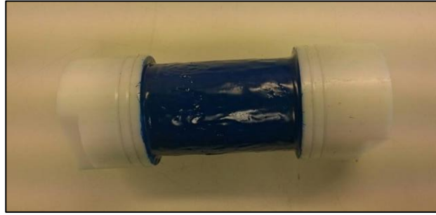
Figure 15 – Core plug OMS 1 , prepared with aluminum foil, shrink sleeve, epoxy and end pieces.
