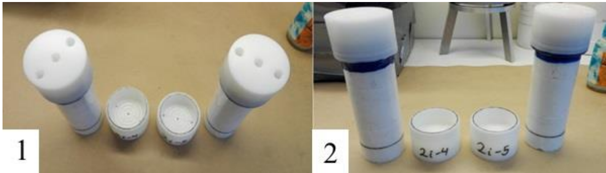
Figure 7-5: The top end-pieces are attached with epoxy, and the bottom end-pieces are ready to be attached to core 2i-4 and 2i-5. 1) Top view where the inside and top of the end-piece can be seen. 2) Side view where the epoxy attaching the end-piece to the core is seen. The black lines mark the overlap of the end-pieces on the bottom core segment.
