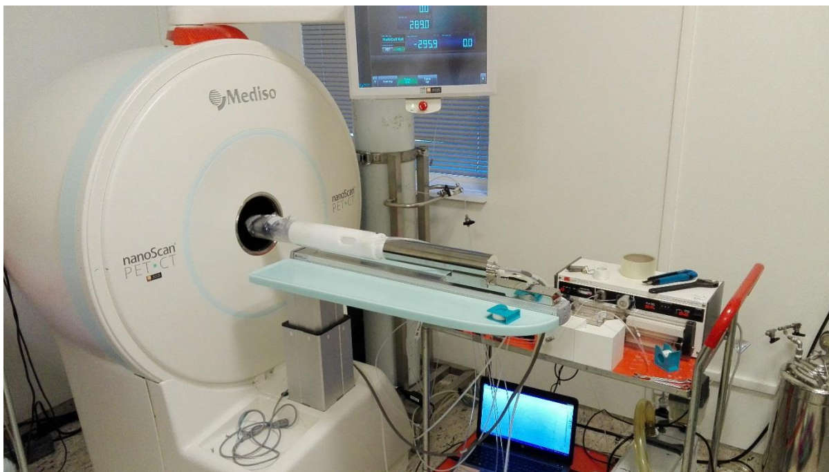
Figure 10-2: Experiments were done inside a PET/CT -scanner. The fractured core was placed on a modified "bed" originally designed for rats. The "bed" with the fractured core was then wrapped in plastic in case of leakage. A leakage inside the PET/CT machine could potentially damage or destroy the machine. All other equipment (pump, pressure transducer, vacuum pump, mas flow controller, laptop, and liquids) was placed on a table next to the PET/CT-scanner and was connected to the core with tubing.
