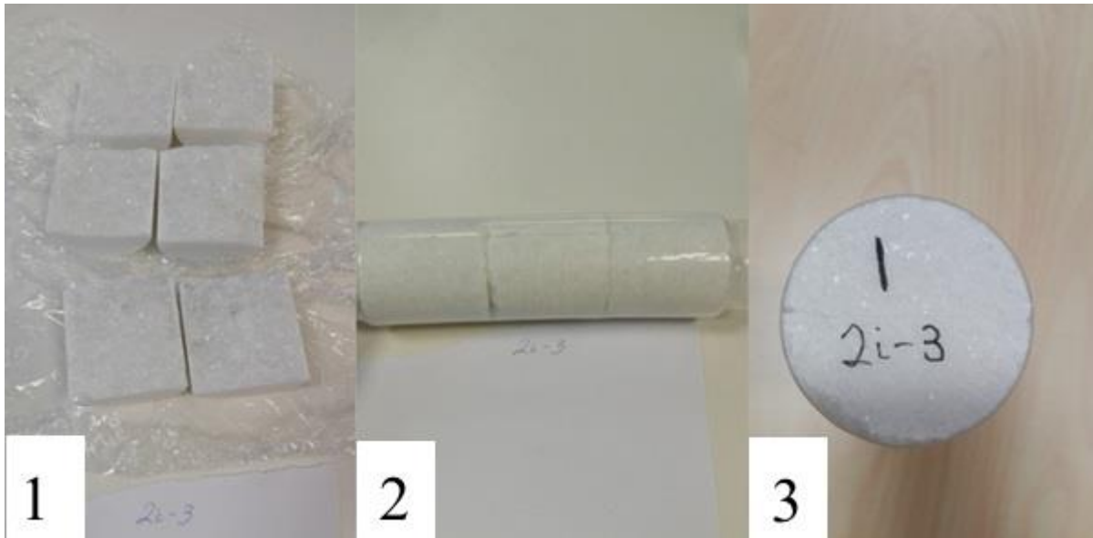
Figure 7-4: 1) The fractured segments of marble next to each other. 2) The segments placed inside the shrink-sleeve 3) Top view of the finished and reassembled core. The fracture is oriented horizontally on this picture between the “1” and “2i-3”.
