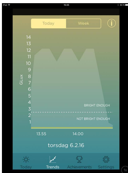
Figure 14: Data available from SunSprite app. The graph shows illuminance in "GoodLux", GLux, on the vertical axis, and time in hours and minutes on the horizontal axis. Notice the cut of on the graph at about 12 GLux.
