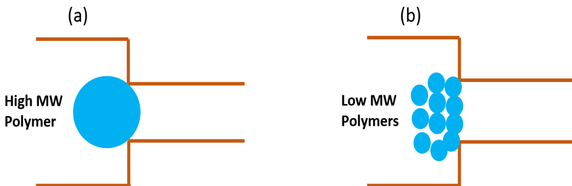
Figure 4.10: Straining (a) of high MW polymers and concentration blocking (b) of low MW polymers relative to pore throats in flow through porous media.
