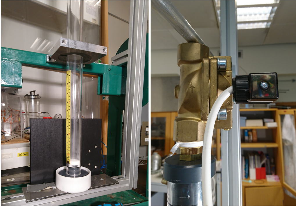
Figure 27: The 40 mm pressure chamber, geometry three, to the left with the solenoid valve to the right.
