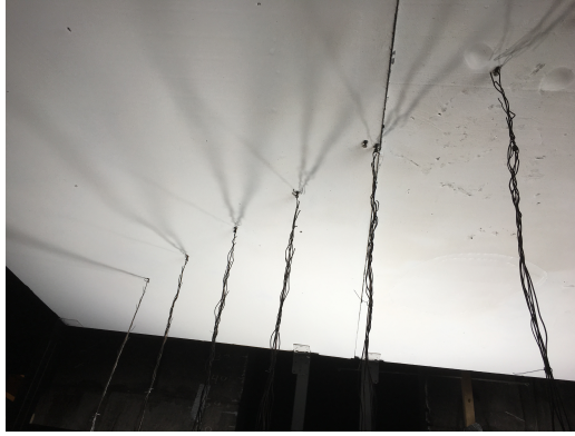
Figure 3.5: Picture towards the roof showing the thermocouple trees, for temperature measurements at different radial positions and distances below the ceiling.
