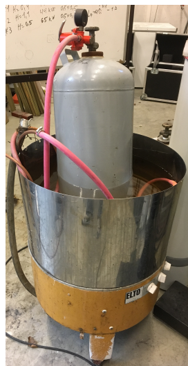
Figure 3.3: Propane gas bottle placed in heating system for optimal performance during the ceiling jet experiments.
