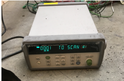
Figure 3.6: Temperature recorder Keysight 34972A Data Acquisition/Switch Unit used for temperature recording in the experiments.
