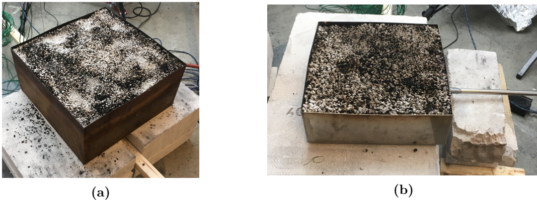
Figure 3.4: Two different sized sandbox burners used in the ceiling jet experiments, with surface area (a) 0.5x0.5 m and (b) 0.3x0.3 m.
