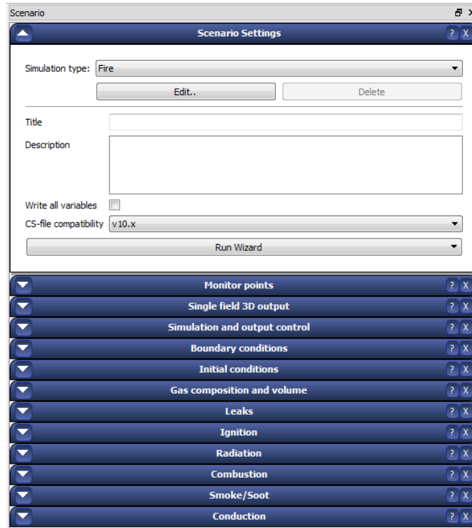
Figure 3.9: Scenario Settings sidebar in FLACS’s pre-processor CASD. The simulation type is set to ‘fire’, displaying the default settings which are usually changed during such simulations.
