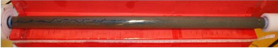
Figure 20: Picture of imbibition tube SP13 after spontaneous imbibition has finished, the inlet side is to the left. The tunnel created during the absolute permeability measurements is completely saturated with dyed mineral oil (Decane).
