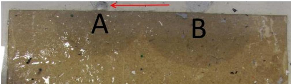
*Figure 34: Spontaneous imbibition into a two-dimensional model with two open areas, Onset 20. The arrow points at a bubble of produced air at the A side inlet. The A imbibed area is smaller than the B imbibed area. The picture is taken 1 hour and 7 minutes after the experiment was initiated.*
