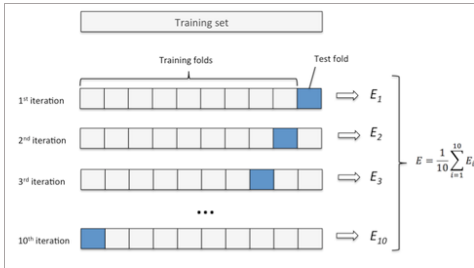
Fig. 3-5 10-fold cross validation. The designated training set is further divided up into K folds ( K=10 ), each of these will now function as a hold-out test set in K iterations. Finally, the scores obtained from the model on individual iterations are summed and averaged into the final score. (image source: https://sebastianraschka.com )
