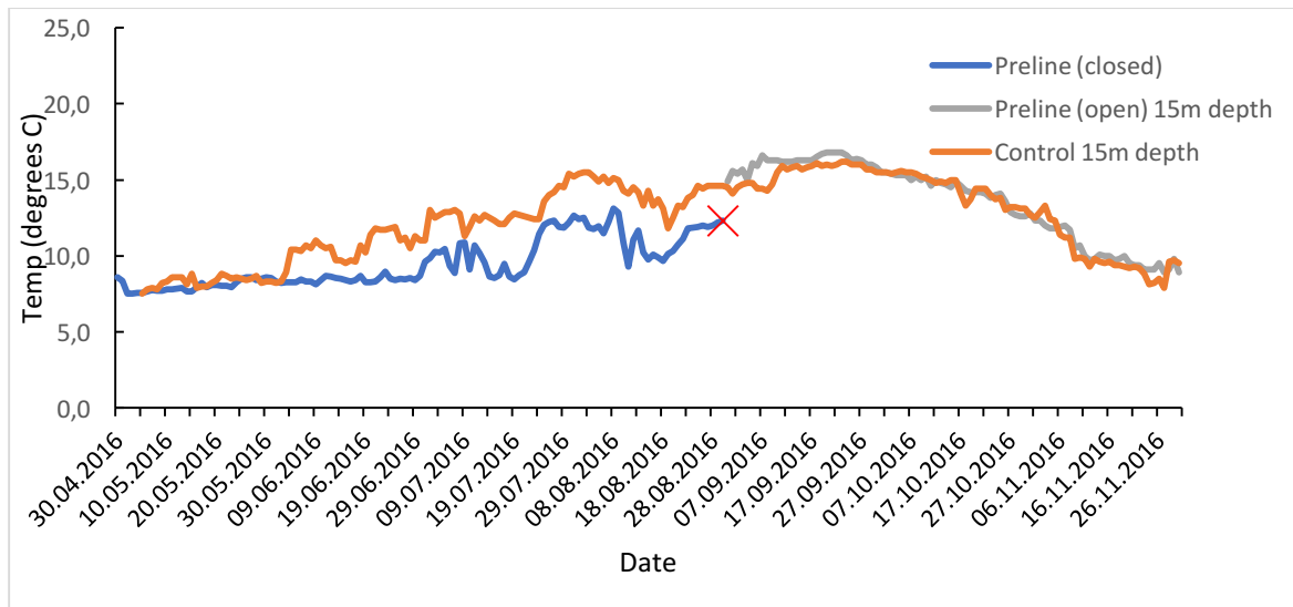
Figure 6.5: Temperature in the Preline system (blue), (water taken from 35 m depth), up until transfer to open net pen located at Buholmen (31.08.16), and thereafter the temperature at Buholmen at 15 m depth (grey). Orange line shows temperature at the Control facility at 15 m depth throughout the whole period.
