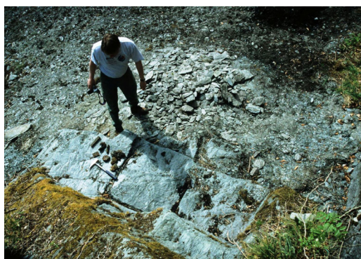
Figure 14. A quarry floor at the Netteland chlorite schist quarry area exposing worked channels for extraction of square blocks. (Photo: Ø. J. Jansen).
