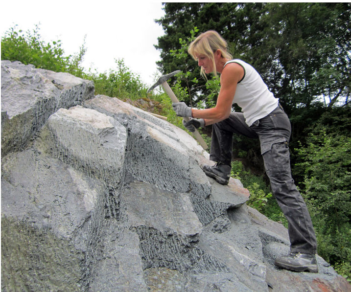
Figure 6. The soapstone quarry as a workspace, as a cultural and social space. Eva Stavsoien experimenting with extraction of ashlar in the Klungen soapstone quarry (Øysand quarry landscape) by Trondheim. The picture gives a fairly good idea of how work was carried out in a medieval soapstone quarry aimed for production of building stone. (Photo: P. Storemyr).
