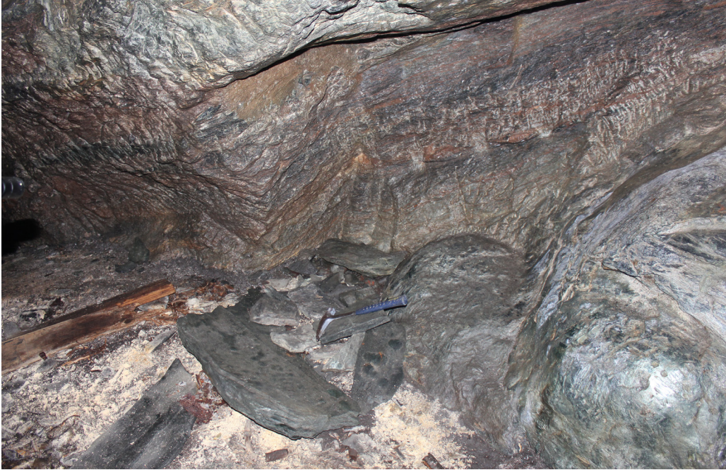
Figure 11. Tool marks made by heavy iron picks at the base of the western quarry wall of Baldersheim soapstone quarry show extraction of large ashlars. The exposed soapstone has a banded appearance due to layers and lenses containing variable amounts of chlorite, talc and carbonate. (Photo: Ø. J. Jansen).
