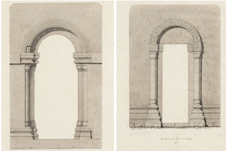
Figure 5. Right: The south portal of the medieval chancel of Alstahaug church with the round-headed arch with the sunken star pattern carved in soapstone. Left: The opening between the medieval chancel and nave. Drawings by C. Christie in 1860 before the church was rebuilt in 1863–65. (©The Directorate for Cultural Heritage, The Archive).
