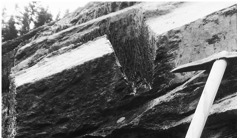
Figure 6. The slanting channel walls resulting in blocks with a larger bottom than top side. (Photo: E. Stavsoien & H. Grøtt).
