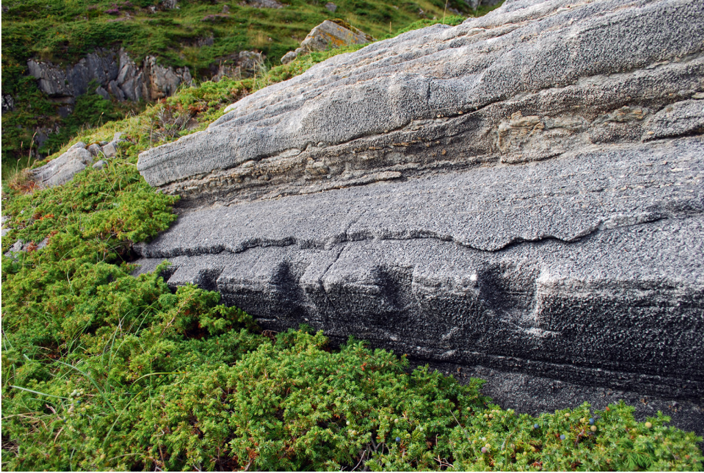
Figure 16. Part of the substantial medieval marble quarry at the island of Allmenningen off the coast of Central Norway, some 140 km north of Trondheim. This quarry produced about 10.000 marble shafts in the Middle Ages. Wedge holes for splitting blocks can be seen on the picture. (Photo: P. Storemyr).
