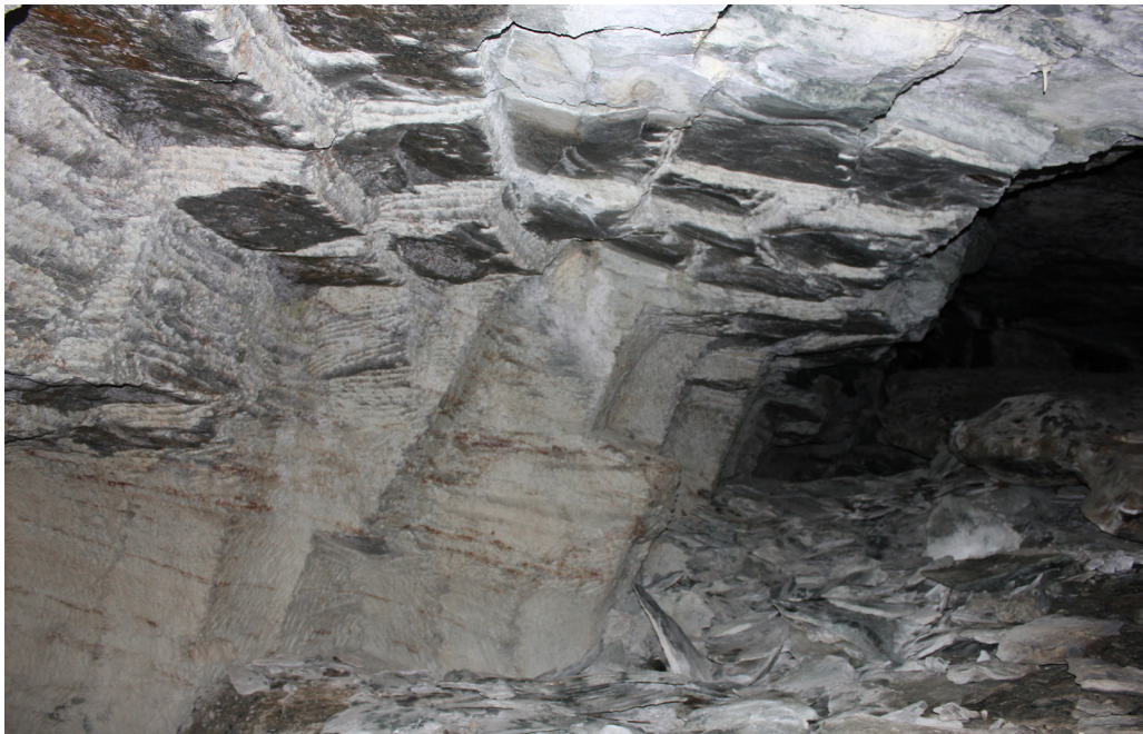
Figure 13. Bakkehidlaren chlorite schist quarry. The quarry marks and angular corners at the base of the quarry wall imply the production of slabs and ashlars, while the pick and chisel marks in the ceiling are related to extraction of square flagstone – probably for roofing purposes. (Photo: Ø. J. Jansen).
