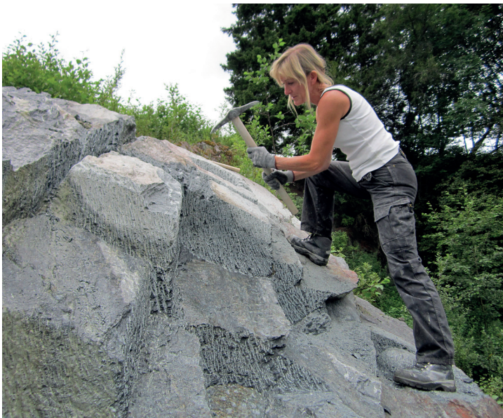
Figure 6. The soapstone quarry as a workspace, as a cultural and social space. Eva Stavsjøien experimenting with extraction of ashlars in the Klungen soapstone quarry (Øysand quarry landscape) by Trondheim. The picture gives a fairly good idea of how work was carried out in a medieval soapstone quarry aimed for production of building stone. (Photo: P. Storemyr).
