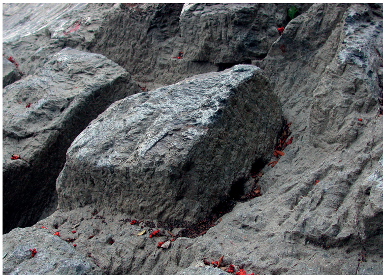
Figure 9. Close-up of an excavated part of the Bakkaunet quarry, prior to the building of an apartment complex by 2005. Soapstone block with carved-out wedge holes. (Photo: P. Storemyr 2004).
