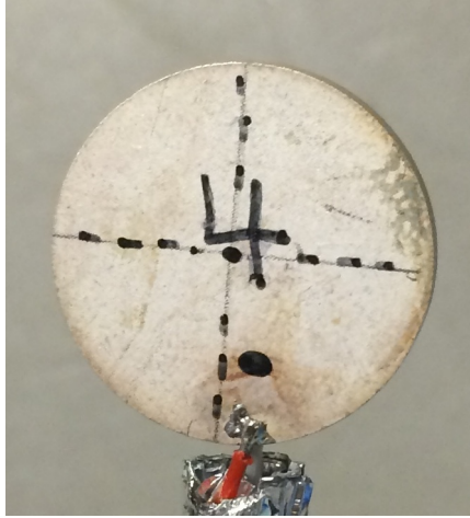
Figure 4.3: Closeup of a transducer inscribed with a reticle.
