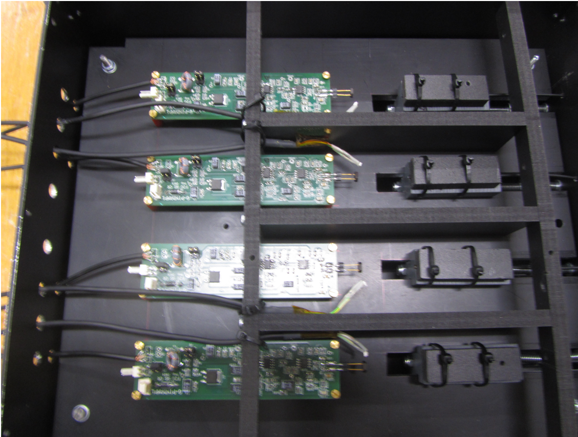
Figure 2.1: Here we see the internal layout of the black boxed used in the analysis. The four pre-amplifiers can be seen with their own SiPM mounted in the socket. The small white chip seen near the detectors is the PT1000 temperature monitors. The cable ties seen on the right hand side in the picture are there to securely fasten the mounting for the optical fibers.
