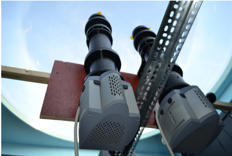
Figure 4.4: The two MOOSE all-sky imagers mounted in the same dome. One captures the green aurora (557.7 nm), and the other captures the violet-blue aurora (427.8 nm). Photo by Robert Michell.
