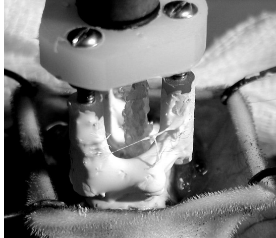
Figure 14.2: Attaching the platform to the skull. The platform can later be adjusted up or down by tightening the screws seen on top of the picture.
