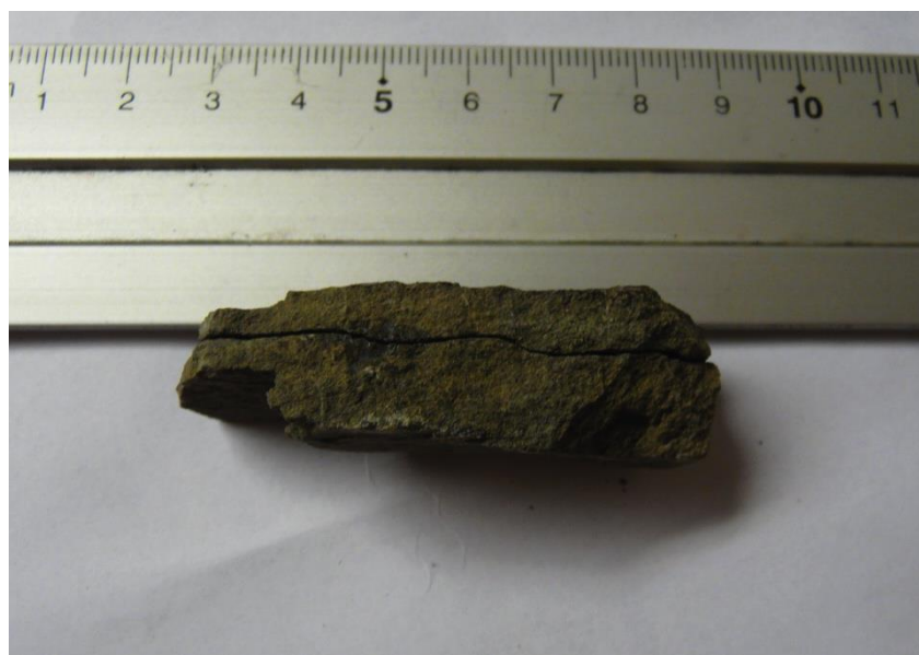
Figure 4.7: Facie M 1 sample with small-scale undulations and weak lamination.
