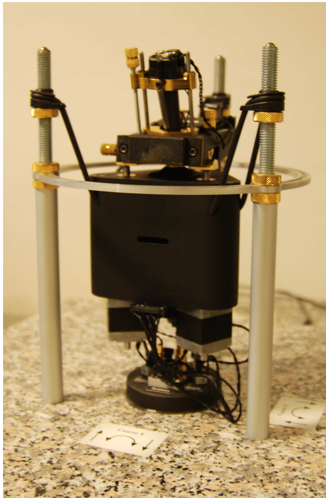
Figure 3.3: Anfatec "Eddy" atomic force microscope intended for educational purposes, and used for simple height measurements.
