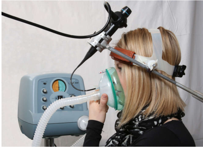
Figure 5. The set up in Study #I with laryngoscope going through a modified interface and attached to a custom made headset.
