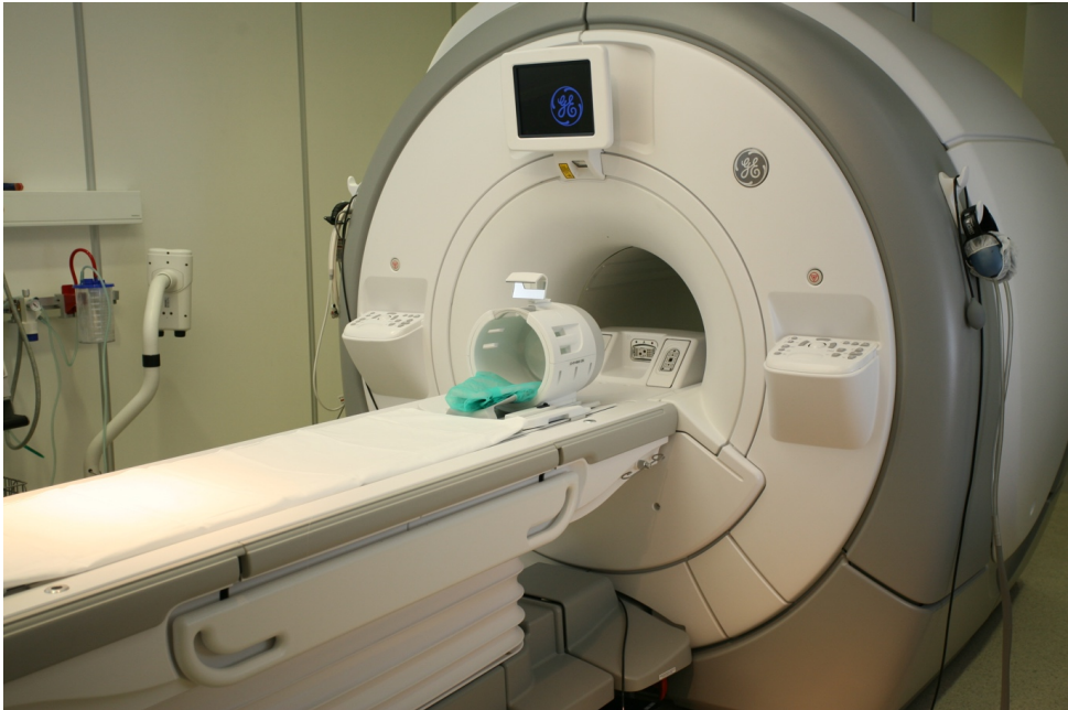
Figure 1: 3.0 T GE Discovery MR750 (Milwaukee, US) with a 32-channel GE head coil. (Photograph by Roger Barndon)
