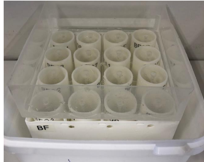
Figure 6.6: Plankton counting chamber used for counting copepodids
