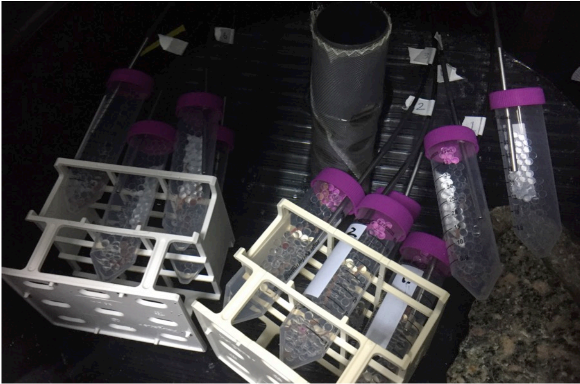
Figure.8 Metabolic experimental set up to determine polychaete respiration rates. X10 chambers all with glass beads and x9 with x5 polychaete individuals of one of three polychaete species. Oxygen measured continually with probe and O 2 sensor on end then stuck through tight hole in lid.
