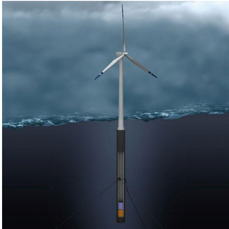
Figure 8. The Hywind concept. [19]
