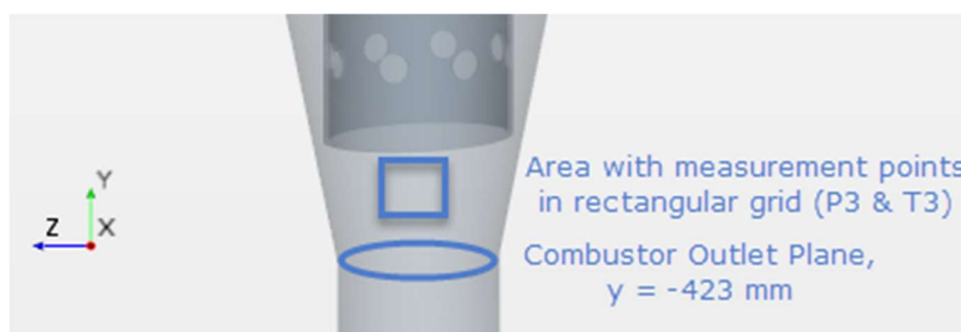
Figure 32: This figure shows the placement of the sampling points used to simulate the placement of measurement points for pressure and temperature on the real combustor. The exact location of P3 and T3 cannot be accurately placed in the model because on the real combustor the depth and angle will vary each time the instruments are mounted. To accommodate for this weakness in the design, a rectangular grid with many points has been set up in the model. These points are separated by 10 mm in all directions from a centre point on the centreline of the combustor.
