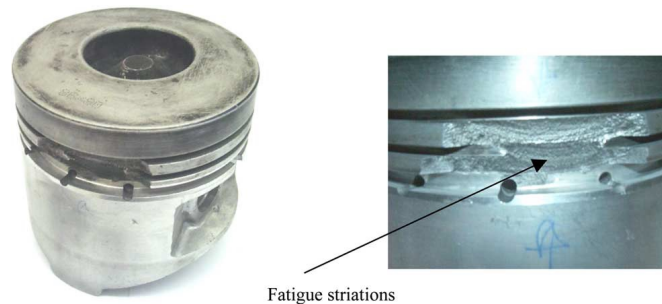
Figure 22: Engine piston with damaged grooves. [30]
