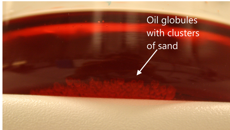
Figure 9.14: Picture taken after sand grains, dyed brine, and n-Decane had been contained in the beaker for 20 minutes. Sand grains were observed in clusters surrounded by oil globules.
