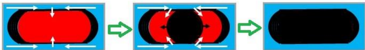
Figure 4.15. The cross-sectional schematic of gas consumption (red) encapsulated by hydrate (black). Water (blue) migrates through wetting water films and permeates through the thinner hydrate films/shell in the pore center (white arrows). Gas is consumed in the pore center. As a result, crystalline hydrate develops in the pore center and further gas consumption continues towards the pore walls (black arrows) until the gas phase is totally converted to hydrate.
