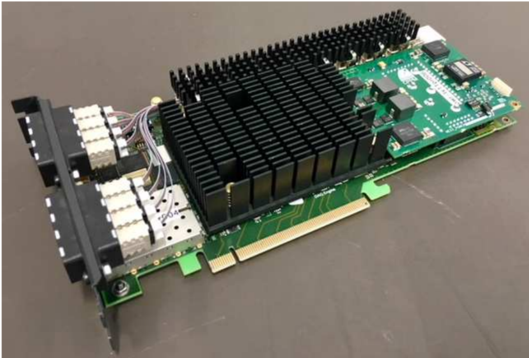
Figure 7: Version 2 of the PCIe40 DAQ board CRU implementation[10]
