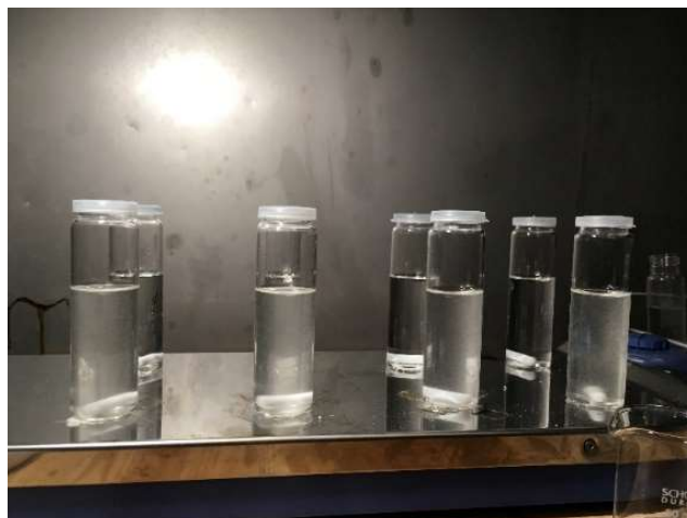
Figure 16. Experimental setup of THF hydrate formation in different chemical environments. Figure shows some of the samples placed on a magnetic stirrer in a pre-cooled refrigerator at desired temperature.
