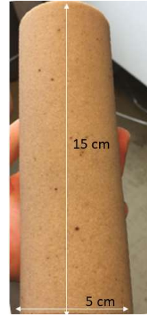
Figure 23. Saturated sandstone core with measurements.
