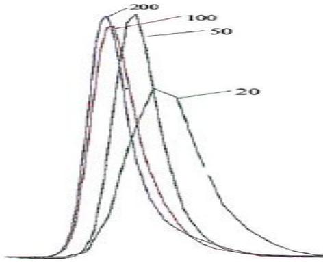
Figure 5 : Effect of data point collection rate on the peak shape at 20, 50, 100, and 200 Hz [24].
