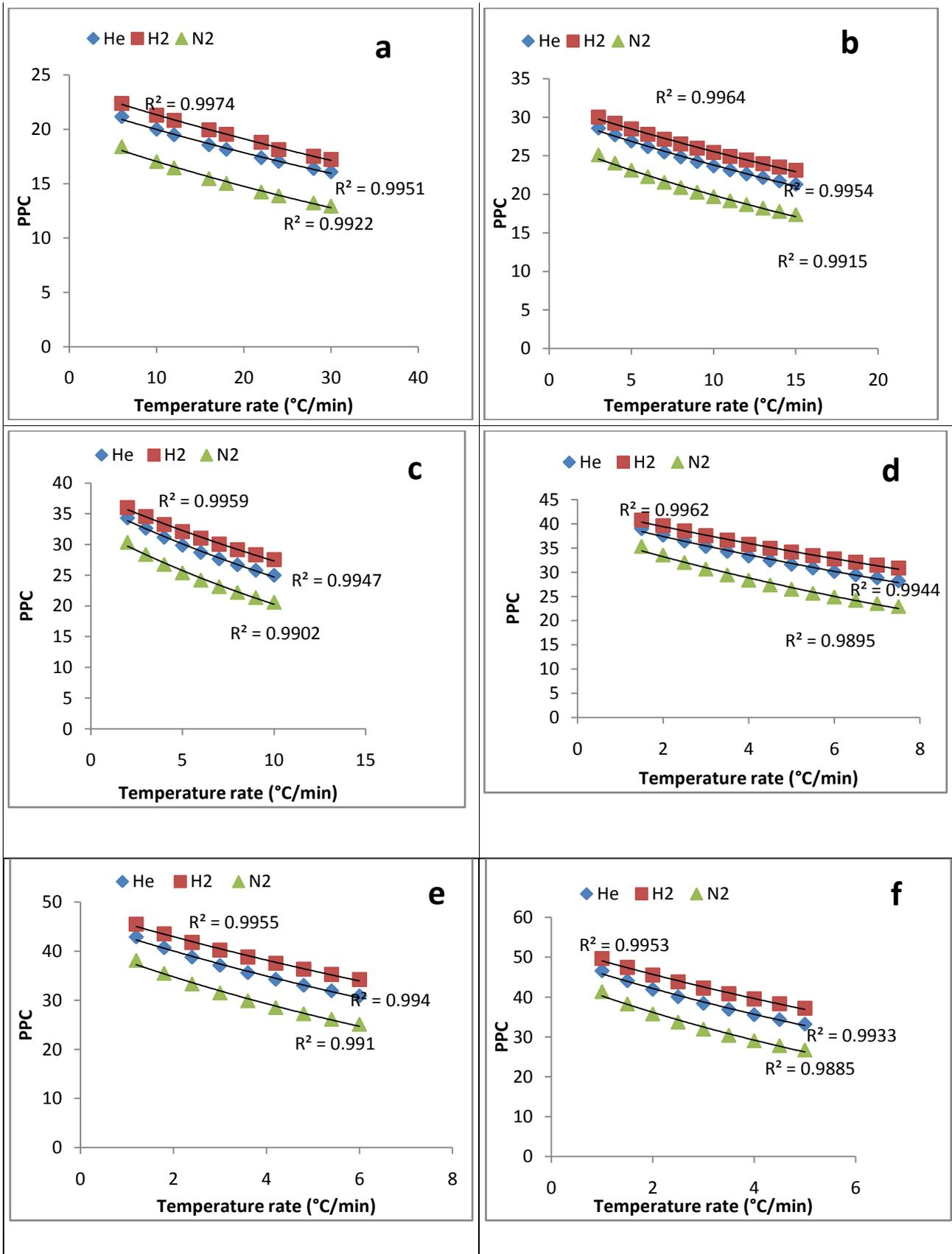
Figure 21: Effect of temperature rate on efficiency column for carrier gases of He, H<sub>2</sub>, N<sub>2</sub> in column length (a) 10m (b) 20m (c) 30m (d) 40m (e) 50m and (f) 60m
