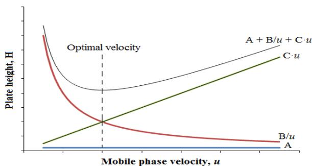
Figure 4: The van Deemter curve
