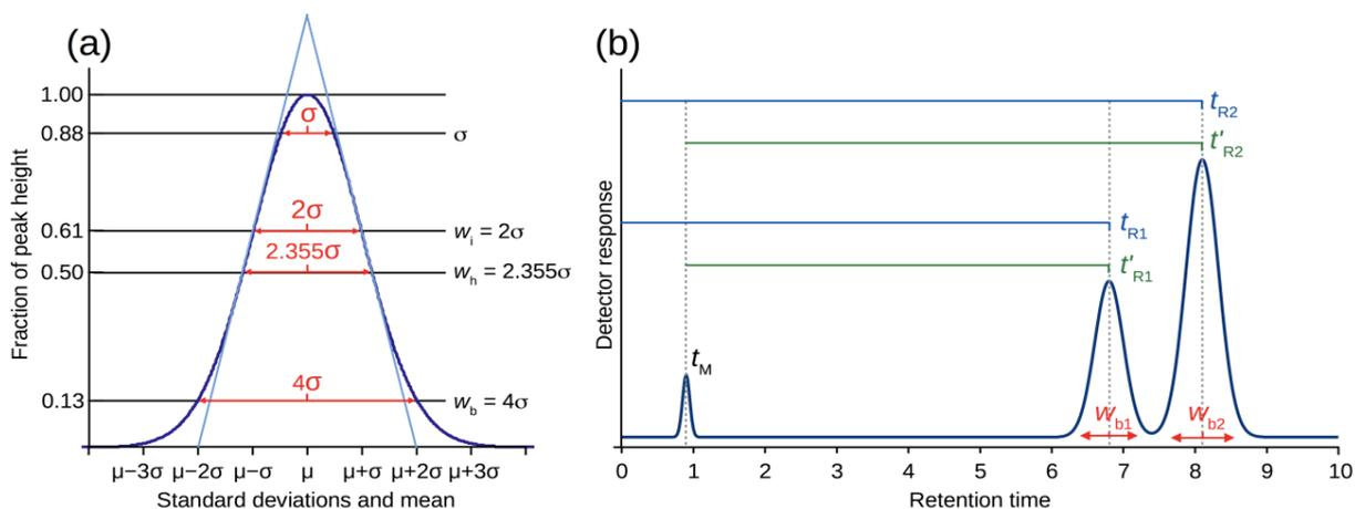
Figure 2: Chromatogram (left) and anatomy of a peak (right)
