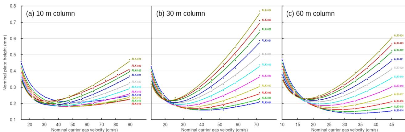
Figure 34: Individual models for alkanes with Helium as carrier gas, (a) 10 m column, (b) 30 m column, (c) 60 m column.
