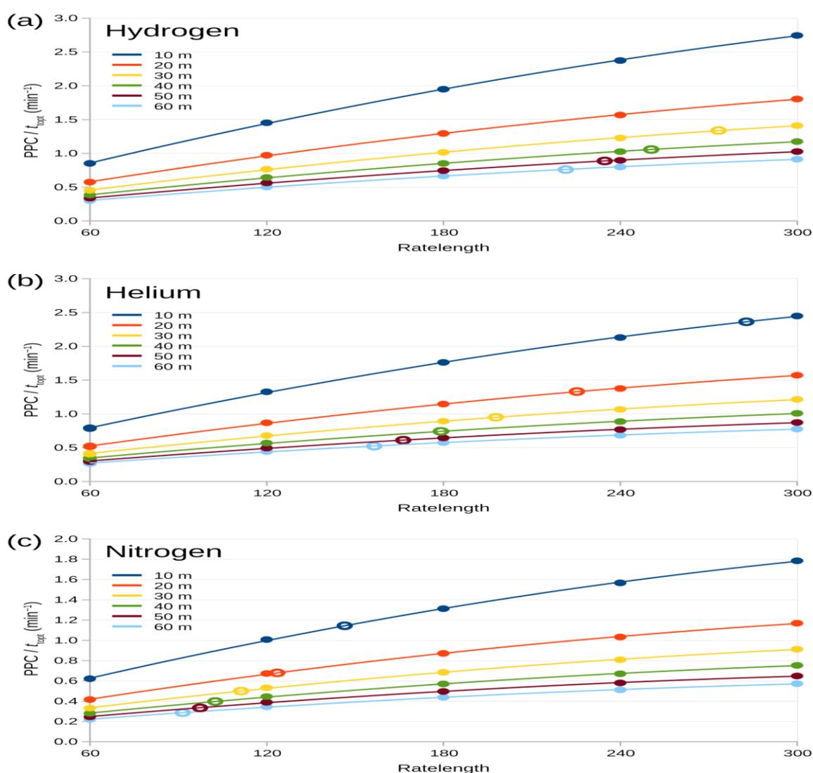
Figure 23: Plots of  $PPC / t_{\text{top}}$  against ratelength for different column lengths and the three different carrier gases, hydrogen (a), helium (b) and nitrogen (c). Open circles illustrate the proposed optimal ratelengths by the  $10^\circ\text{C}/\text{min}$  criterion (middle estimate).
