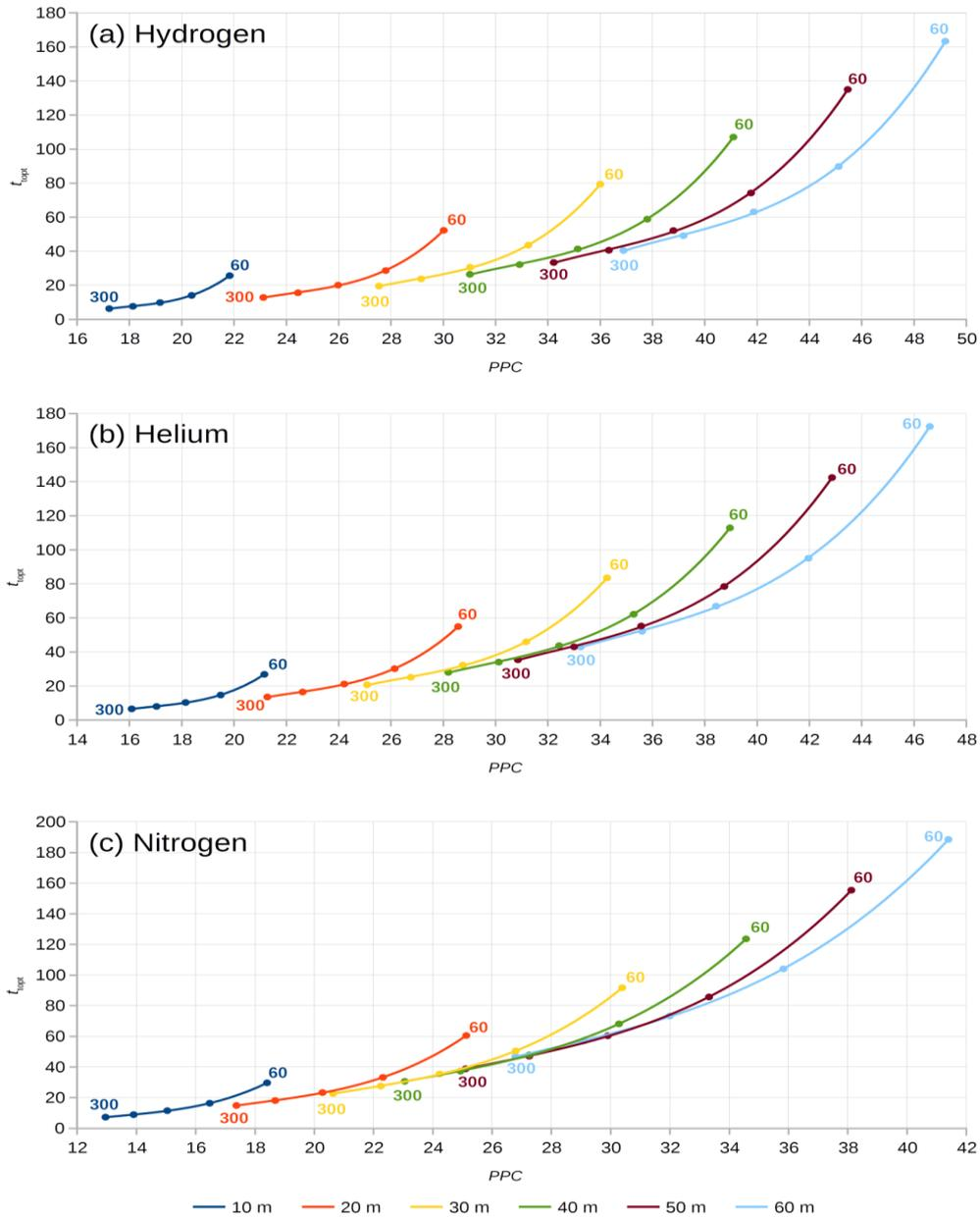
Figure 28: Different column lengths compared for different carrier gases. Numbers on the extremes of the curves show ratelength in  $m^{\circ}C/min$ .
