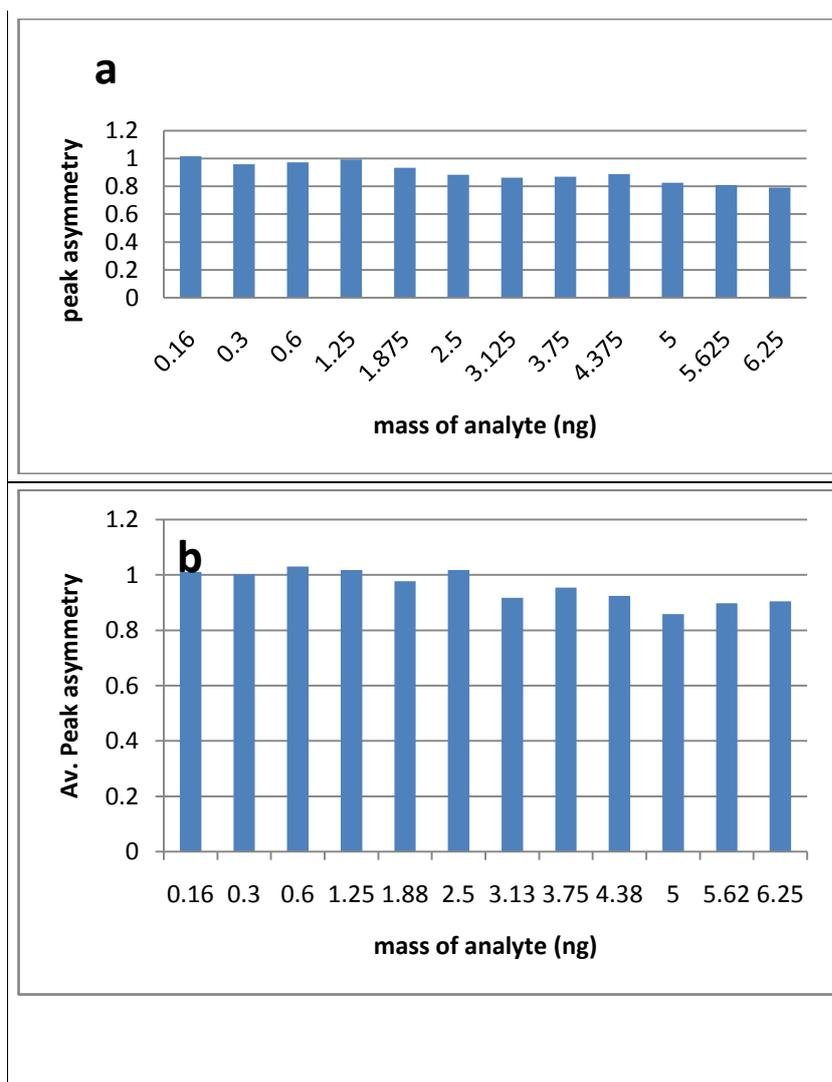
Figure 14: average peak asymmetry at ramp rate (a) 05 °C/min (b) 25 °C/min (HP-5, 10 m x 250  $\mu$ m x 0.25  $\mu$ m, 60 °C for 0 min, 30 cm/s, velocity of carrier gas, He, constant flow rate, 1:40 split ratio)
