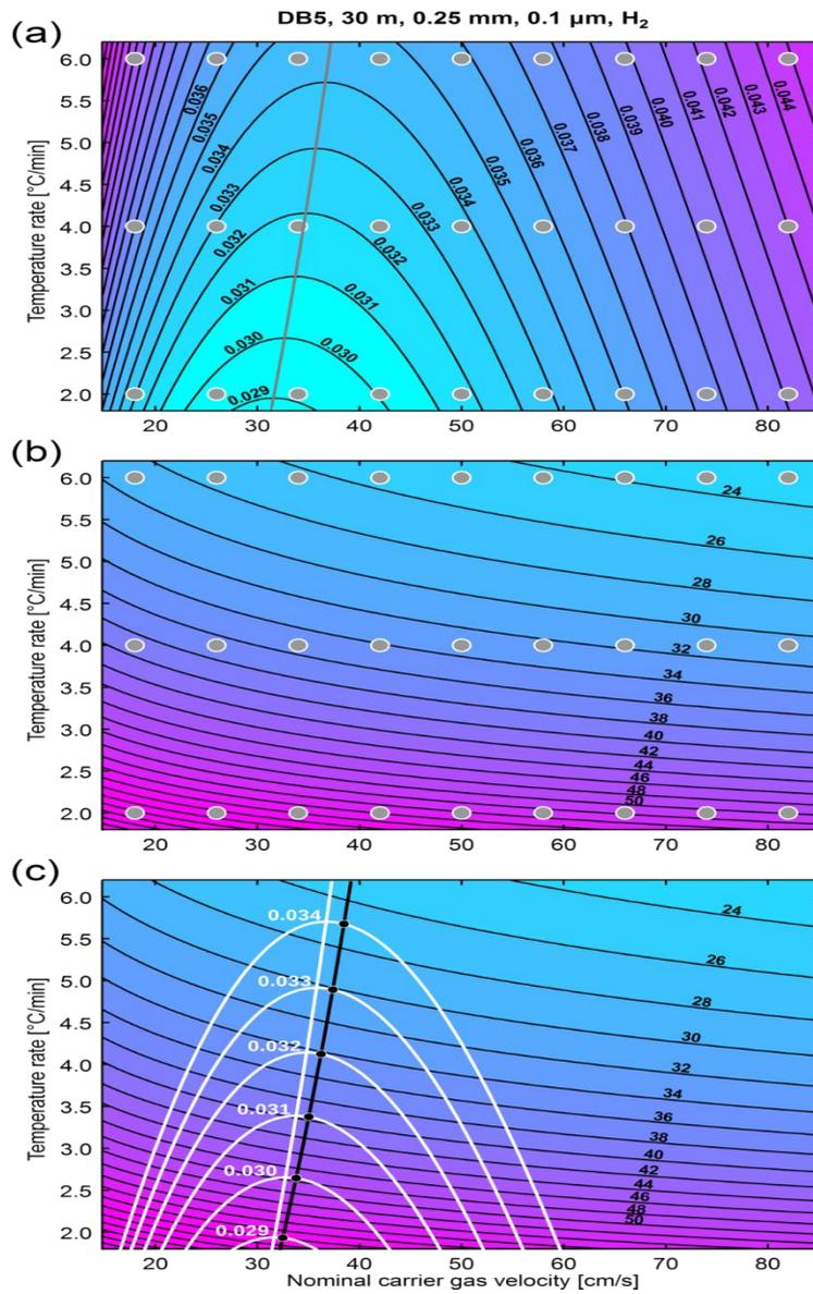
Figure 8: surface response plot a) VD+Int b) log<sub>t<sub>R</sub></sub> c) efficiency – time adapted from [22].
