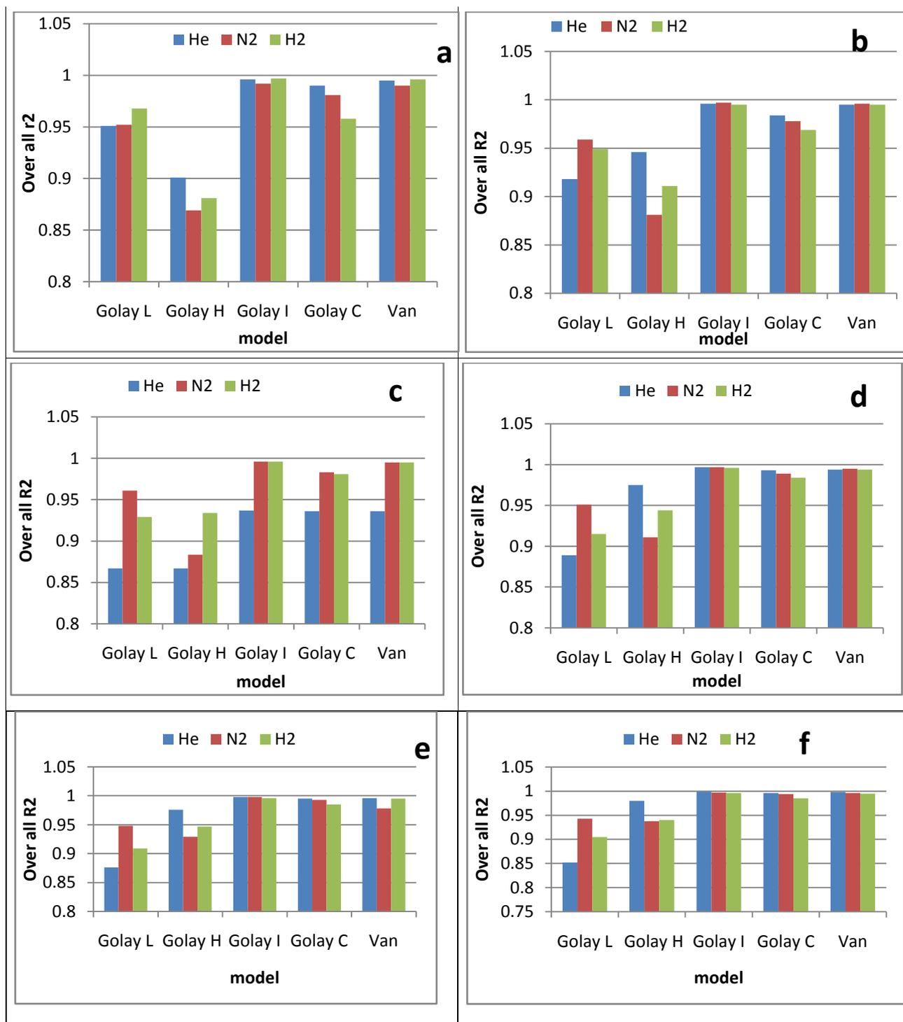
Figure 31: Over all  $R^2$  value of model obtained from He, N<sub>2</sub>, and H<sub>2</sub> as carrier gas in column lengths (a) 10m (b) 20m (c) 30m (d) 40m (e) 50m (f) 60m
