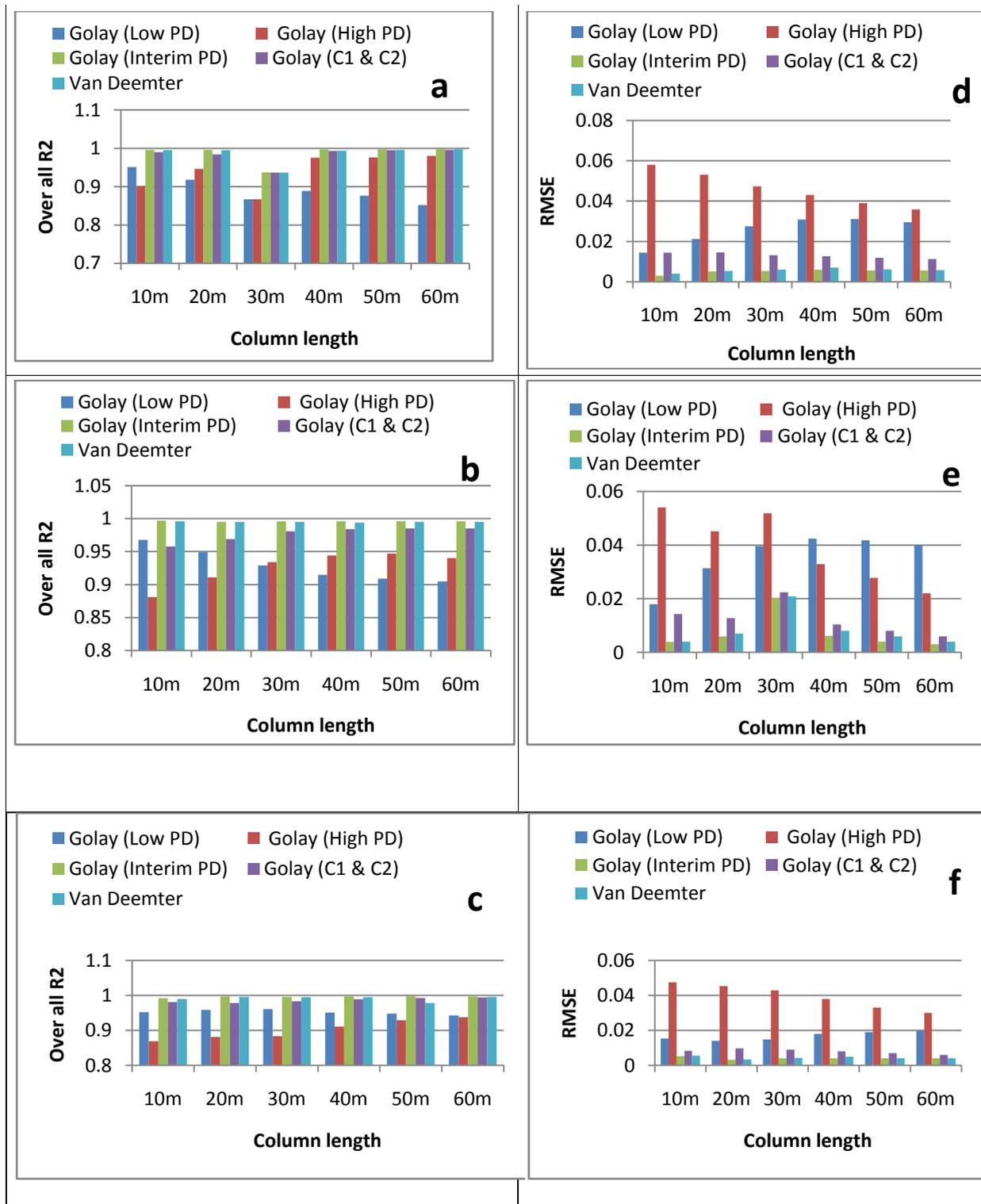
Figure 30: Over all  $R^2$  (left) and RMSE (right) of models obtained with plate height using as (a) Hydrogen (b) Helium (c) Nitrogen and (d) Hydrogen (e) Helium (f) Nitrogen .
