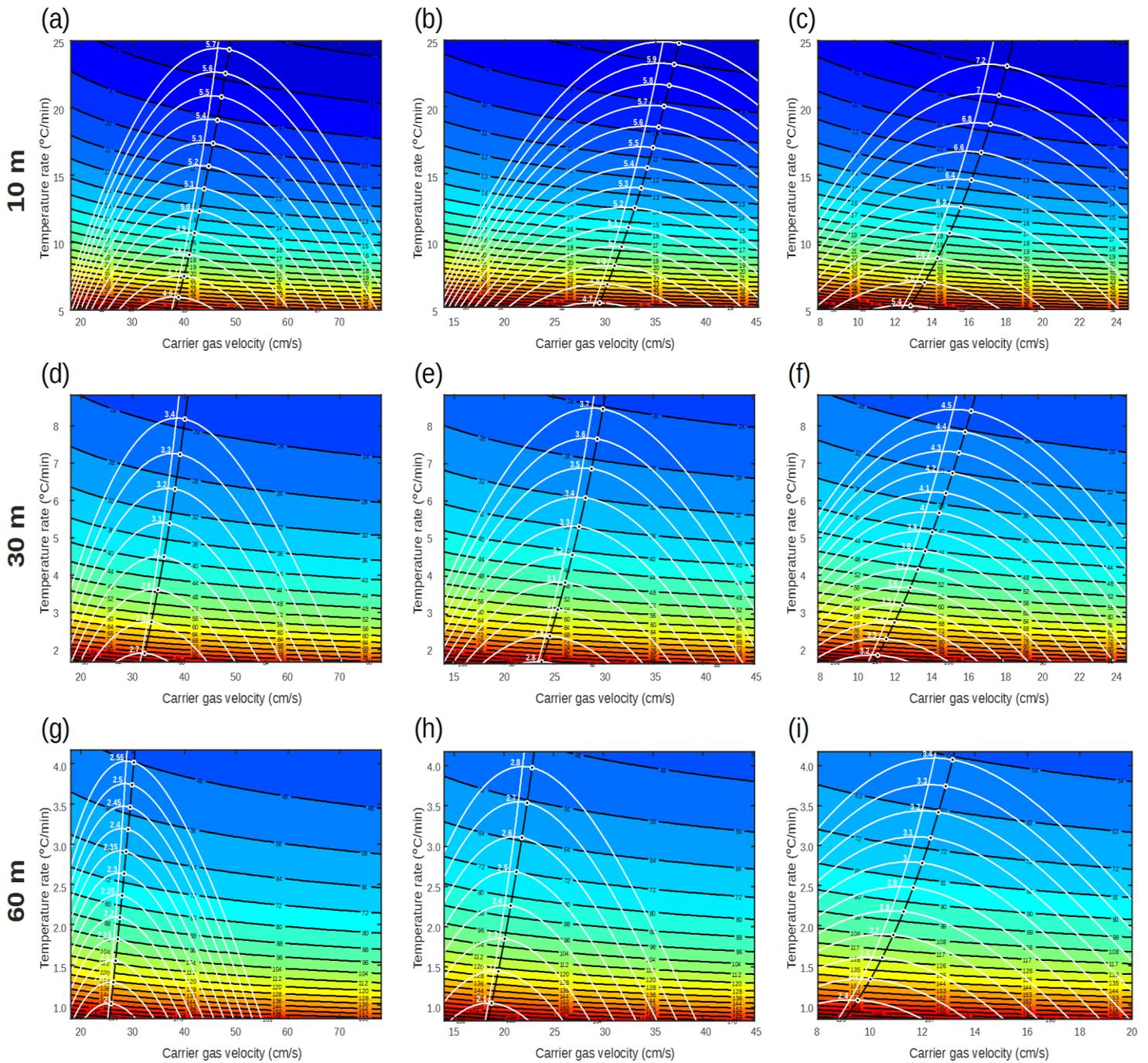
Figure 16: optimal conditions plots for the temperature-programmed pilot experiments
