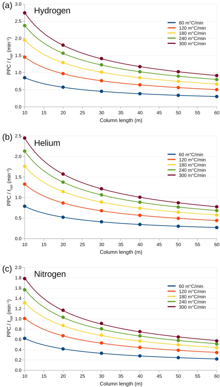
Figure 25: Plots of  $PPC / t_{top}$  against column length for different heating rates and the three different carrier gases, hydrogen (a), helium (b) and nitrogen (c).
