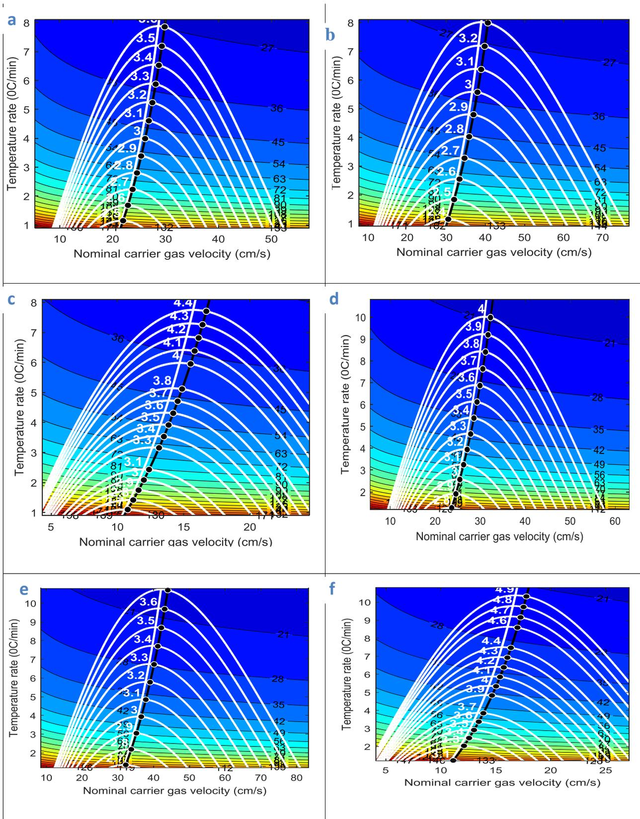
Figure 38: Eff/time obtained from 40m x 250 μm x 0.25 μm, programmed temperature condition in carrier gas (a) He (b) H<sub>2</sub> (c) N<sub>2</sub> and from 30m x 250 μm x 0.25 μm (d) N<sub>2</sub> (e) H<sub>2</sub> (f) N<sub>2</sub>
