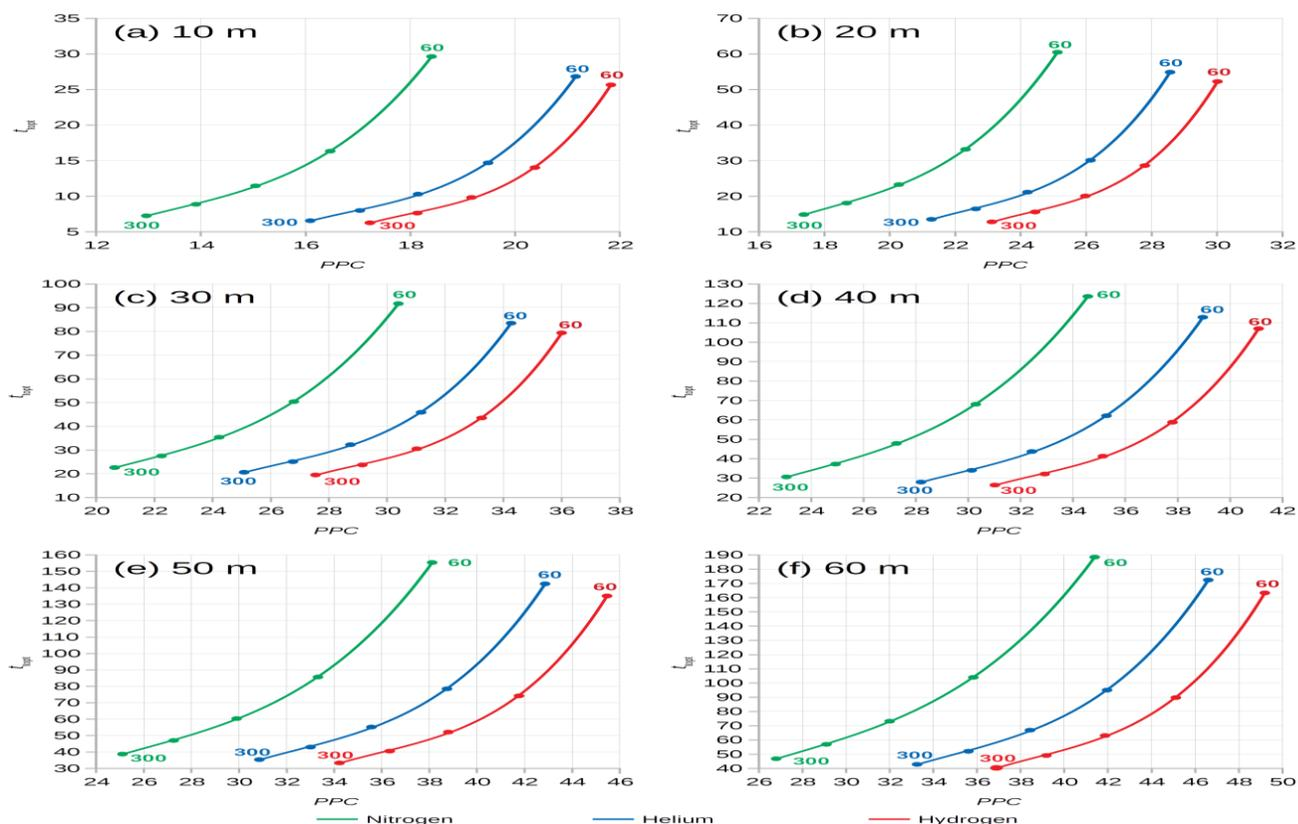
Figure 26: PPC from optimum time for three carrier in the column length a) 10m b) 20m c) 30m d) 40m e) 50m f) 60m. Numbers on the extremes of the curves show rate length in m°C/min.
