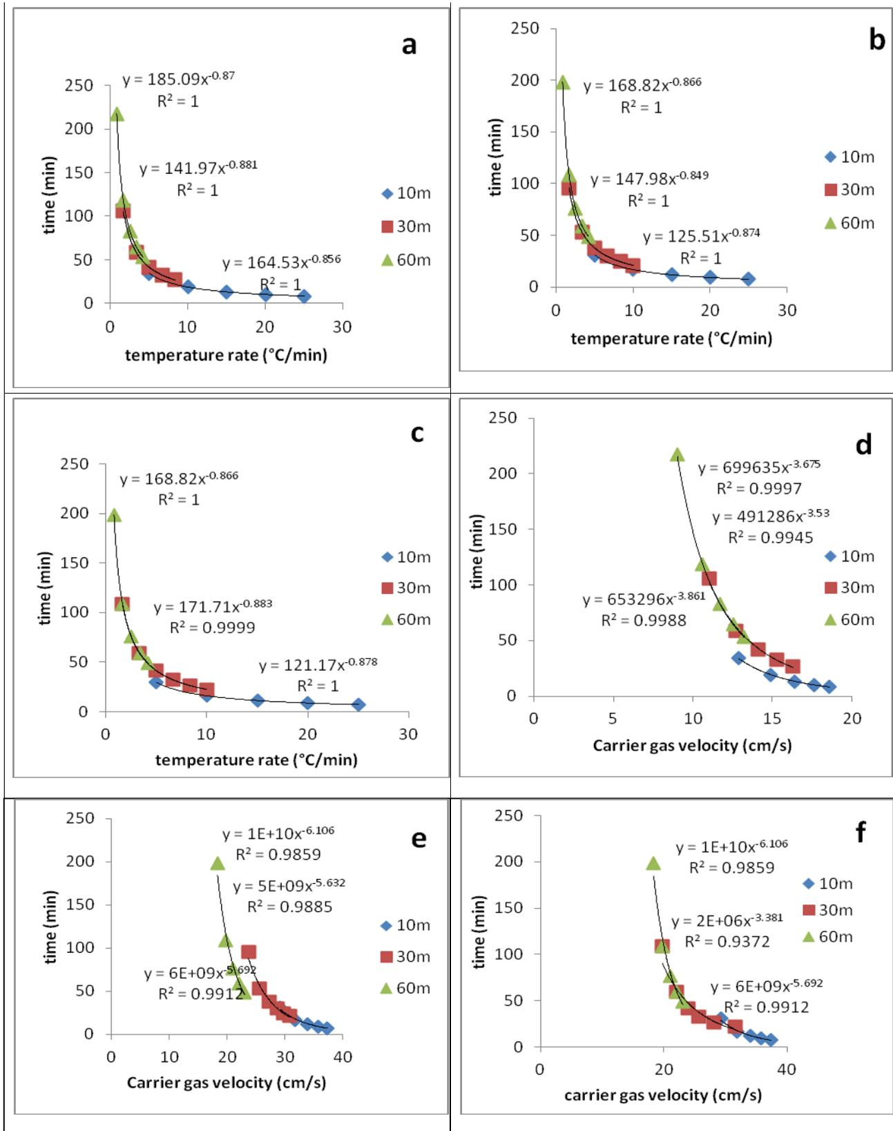
Figure 19: effect of temperature rate and carrier gas velocity on analysis time in three column lengths for carrier gases of (a) N<sub>2</sub> (b) He (c) H<sub>2</sub> and (d) N<sub>2</sub> (e) He (f) H<sub>2</sub> respectively in five level of temperature rate.
