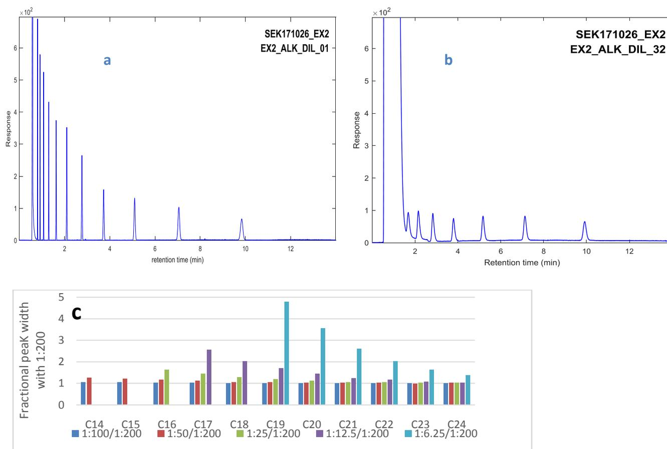
Figure 11: a) Chromatogram of 1:200 split ratio b) Chromatogram of 1:6.5 split ratio c) % of peak width with respect to 1:200 (HP-5, 10 m x 250  $\mu$ m x 0.25  $\mu$ m, 200 °C isothermally, 30 cm/s, velocity of carrier gas, He, constant flow rate)
