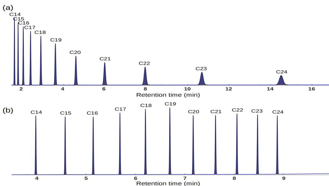
Figure 7: The same C14 to C24 n-alkane mixture analyzed under (a) isothermal and (b) temperature-programmed conditions (data from this work).
