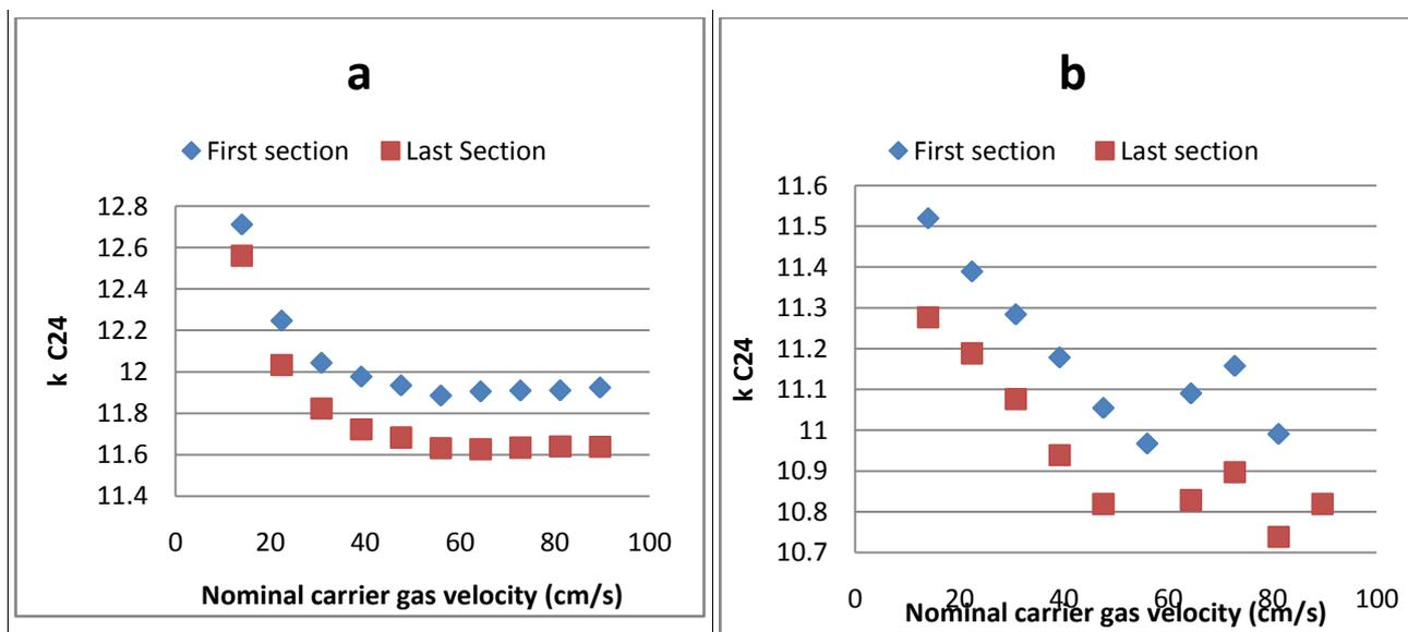
Figure 36: Retention factor of  $C_{24}$  calculated from a)  $t_M$  in cut off 9.05m column length (both in first and last cut off section) and nominal carrier gas velocity b)  $t_M$  based on regression using Chrombox.
