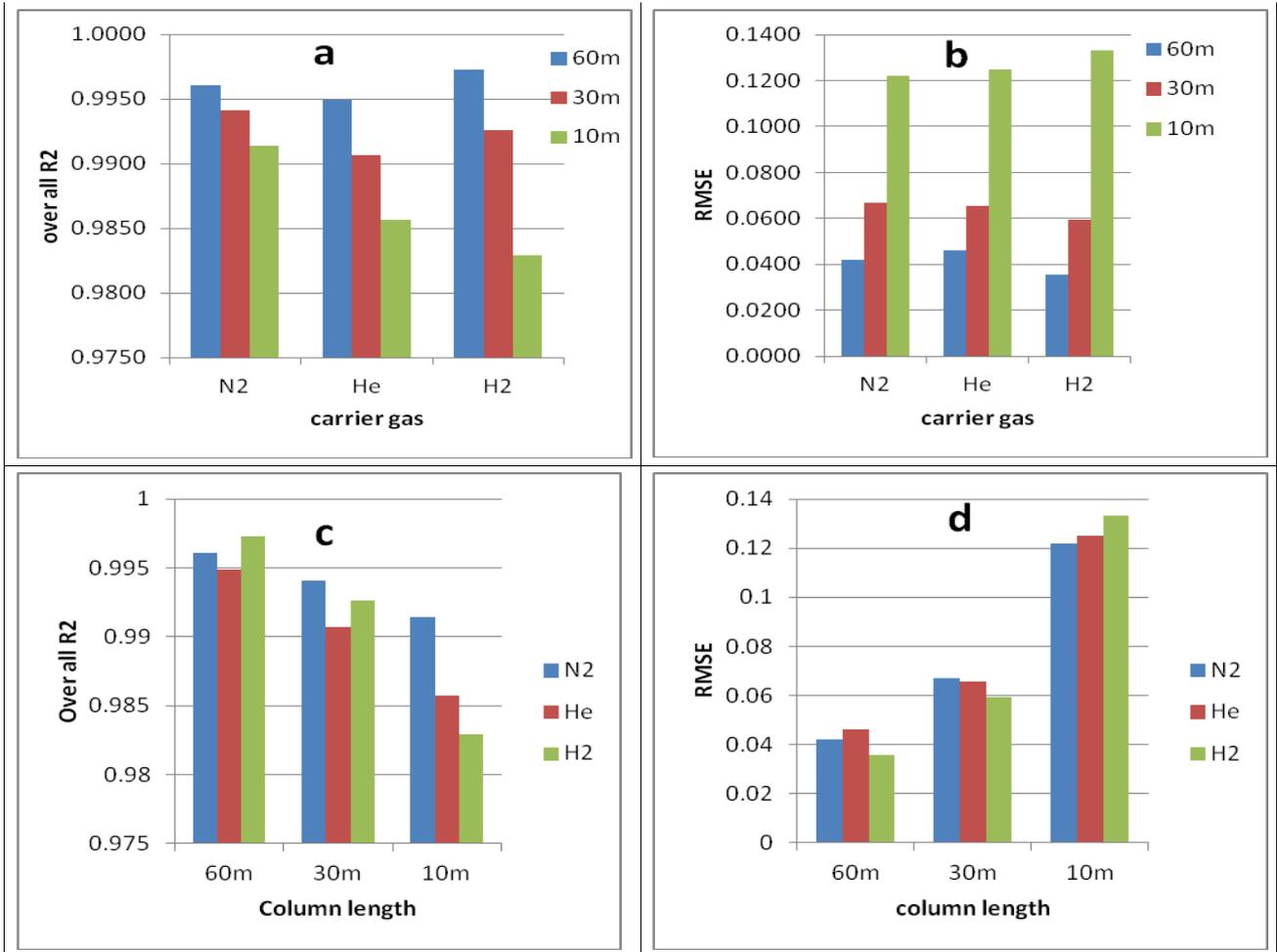
Figure 17 : Overall mean  $R^2$  and RMSE of models obtained from peak width (in five level of temperature rate)
