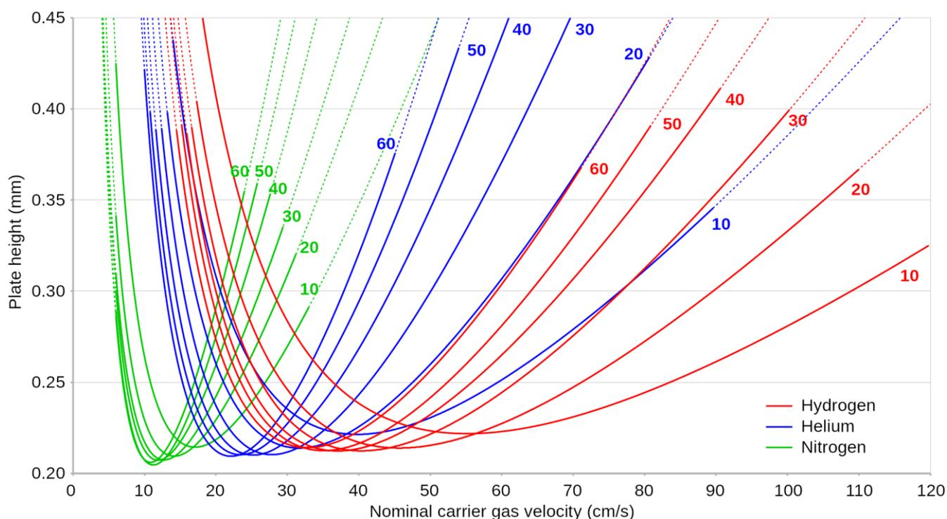
Figure 32: All models for the isothermal experiments based on Equation  $x$  ( $H=B/u^x+Cu^x$ ). Dotted lines show extrapolated regions. The plate height is corrected for the difference between actual and nominal column lengths.
