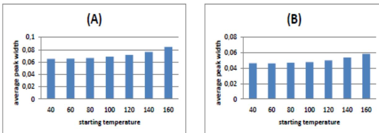
Figure 10 : average peak width at ramp rate (A) 25 °C/min (B) 05 °C/min (HP-5, 10 m x 250  $\mu$ m x 0.25  $\mu$ m, He carrier gas, constant flow rate).
