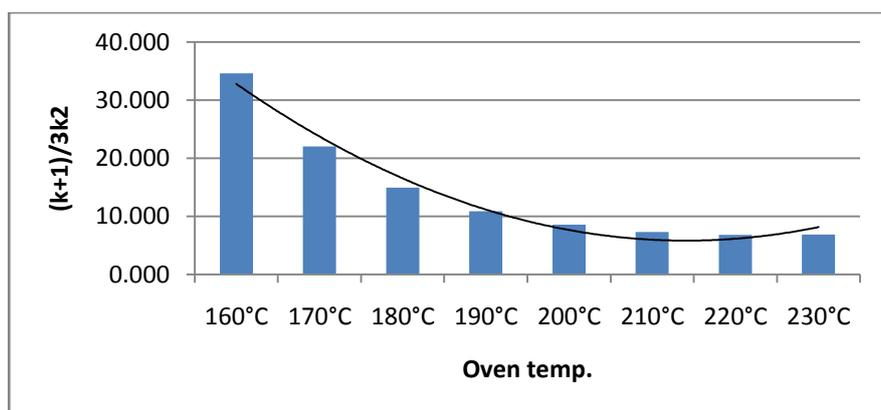
Figure 15: Retention factor obtained from 10m×250µm×0.25µm, He as carrier gas with velocity of 25 cm/s, isothermal condition, 1:200 split ratio, 40 mL/min flow rate of detector gas.
