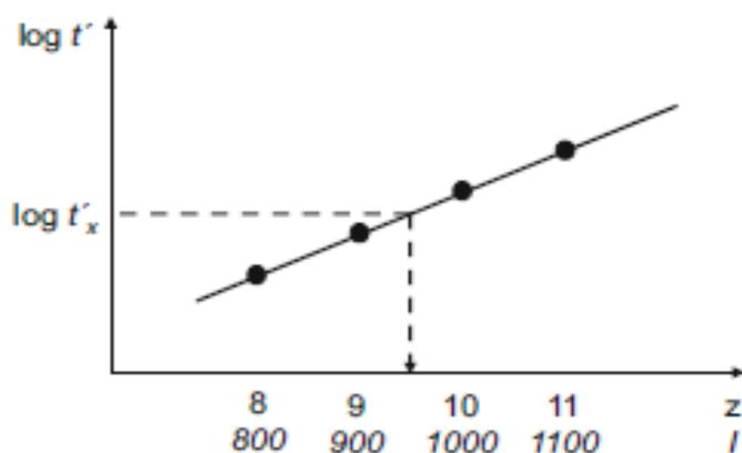
Figure 6: Graphical determination of Kovats retention indices by plotting the log of the adjusted retention time of the n-alkanes against their retention index [21].
