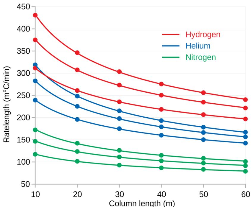
Figure 22: Rate length vs. column length for calculated optimal heating rates using the  $10^{\circ}\text{C}$  per void time criterion.  $u_{\text{topt}}$  at a ratelength of 180 was used as initial carrier gas velocity (low estimate). The three curves for each gas represent velocities at the start (low estimate) at the end (elution temperature of C24, high estimate), and at the middle of the chromatogram (middle estimate). Regression curves are fitted power functions.
