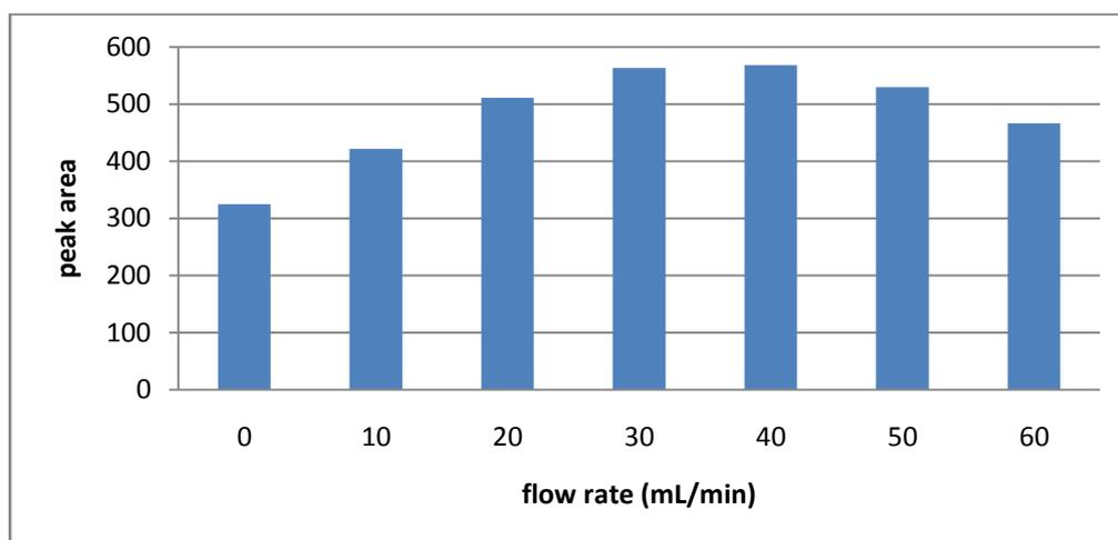
Figure 12: Peak width and Make up gas flow rate (HP-5, 10 m x 250  $\mu$ m x 0.25  $\mu$ m, 60  $^{\circ}$ C for 0 min, 30 $^{\circ}$ C/min, 30 cm/s, velocity of carrier gas, He, constant flow rate, 1:200 split ratio).
