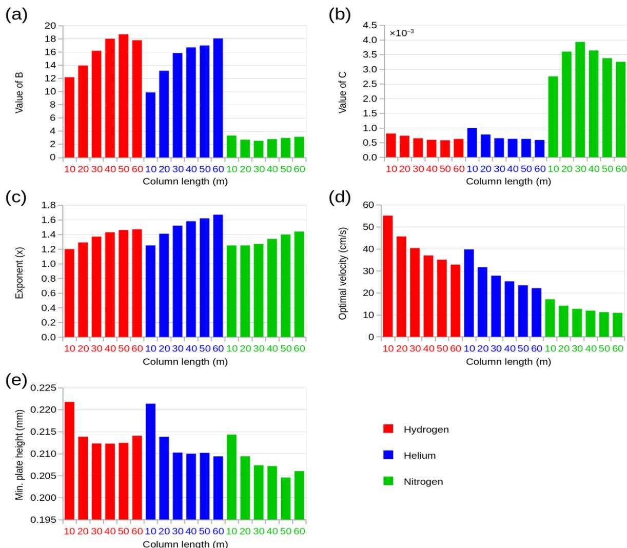
Figure 33: Differences between the models based on Equation  $x$  ( $H=B/u^x+Cu^x$ ). (a) the size of B, (b) the size of C, (c) the size of the exponent,  $x$ , (d) optimal carrier gas velocities, and (e) minimum plate height. The minimum plate height is corrected for the difference between actual and nominal column lengths. Other parameters are not corrected.
