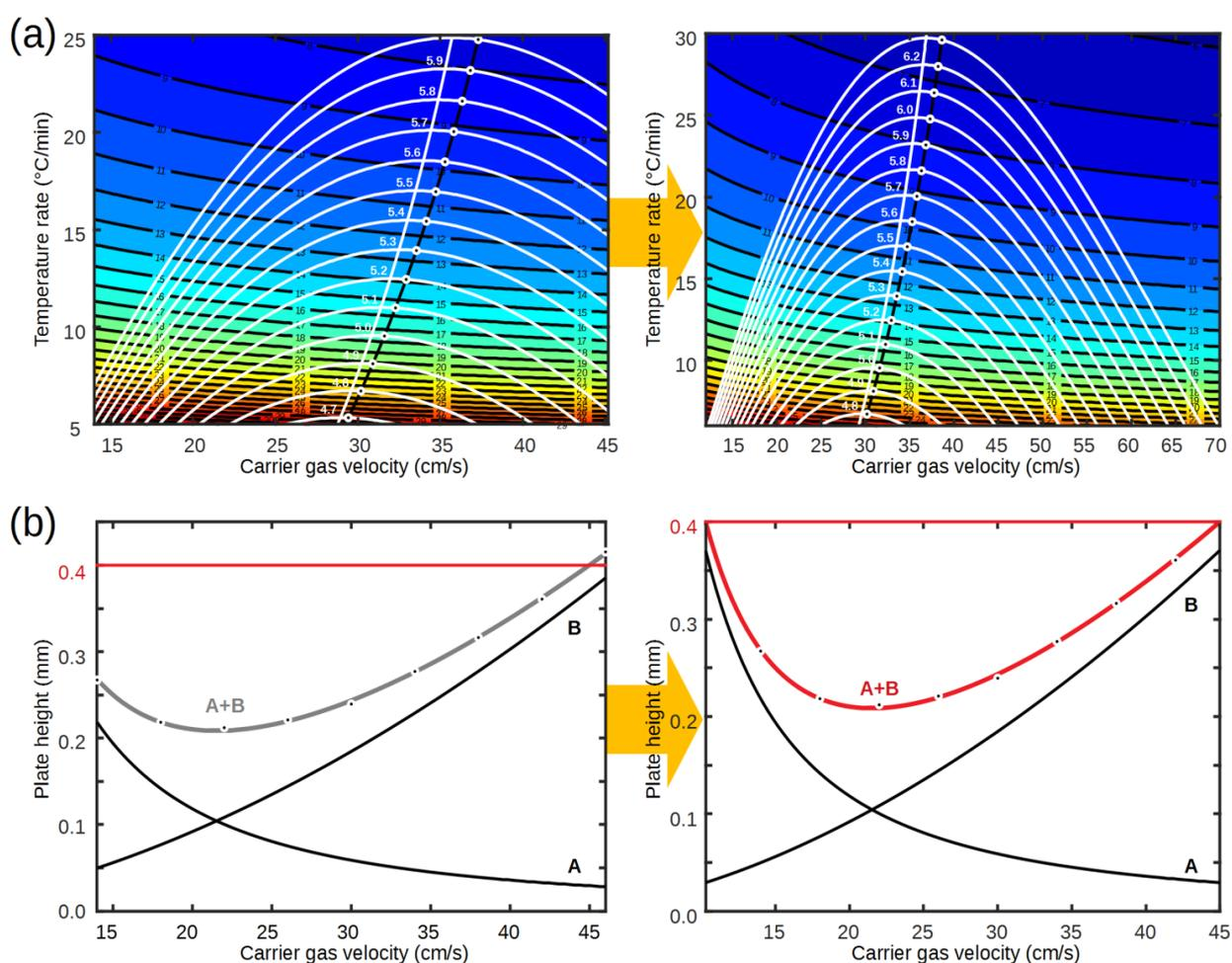
*Figure 20: Standardization of the limits for carrier gas velocities shown for (a) Helium at temperature-programmed conditions and column length 10 m, and (b) Helium isothermal conditions and column length 60 m. The plots to the left shows the model within the experimental conditions, while the plots to the right show the models extrapolated to the limits chosen for the new experiments.*
