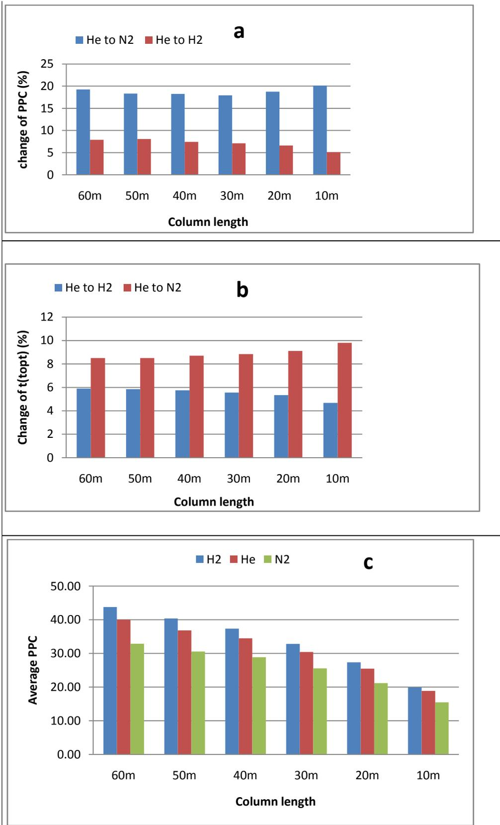
Figure 27: rate of efficiency (a) time (b) when switched one carrier gas over the others. Effect of carrier gas in time-Efficiency (c) in different column lengths (007-5 Quadrex, 10, 20, 30, 40, 50, 60m 250 $\mu$ m $\times$ 0.25 $\mu$ m).
