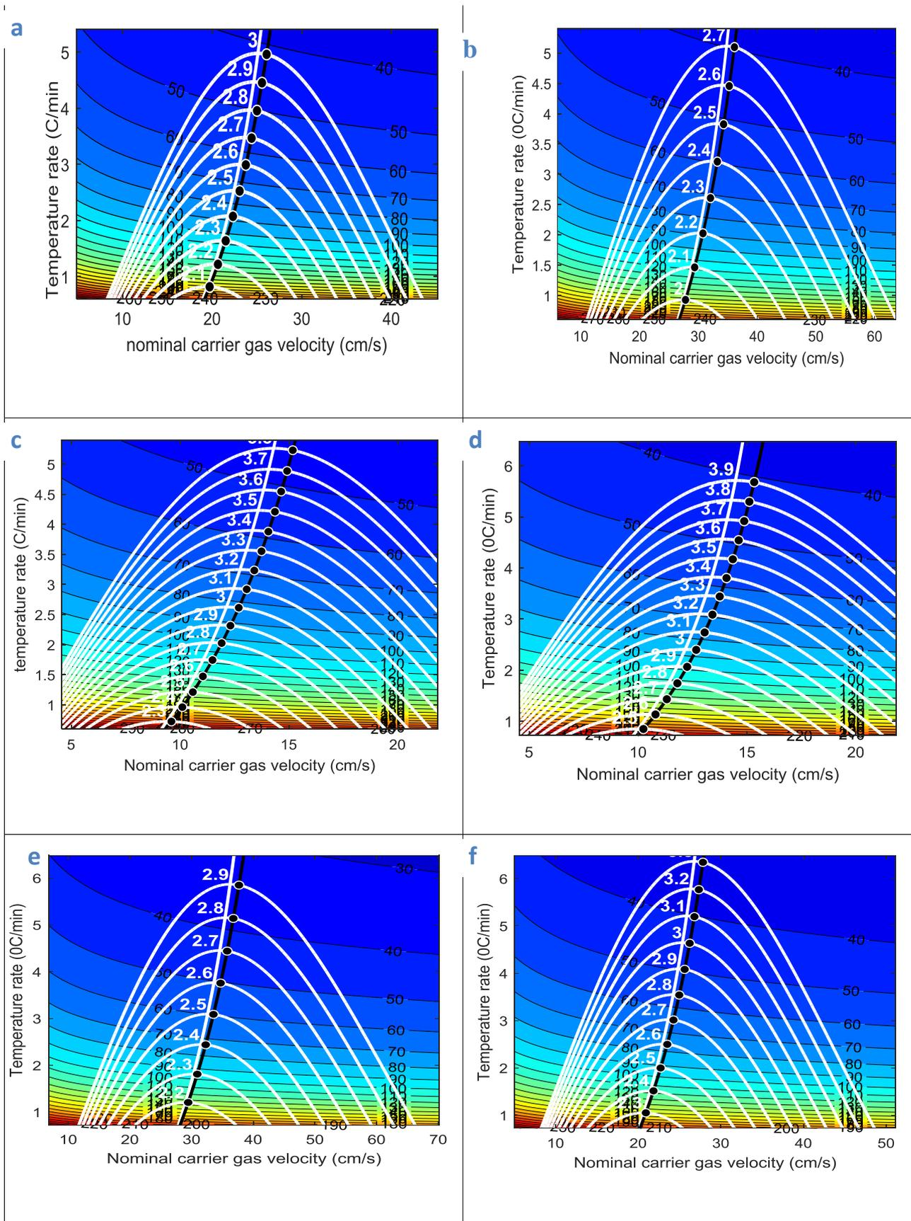
Figure 37: Eff/time obtained from 60m x 250 μm x 0.25 μm, programmed temperature condition in carrier gas (a) He (b) H<sub>2</sub> (c) N<sub>2</sub> and from 50m x 250 μm x 0.25 μm (d) N<sub>2</sub> (e) H<sub>2</sub> (f) N<sub>2</sub>
