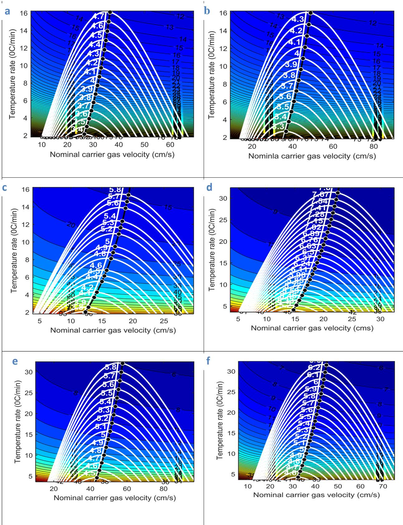
Figure 39: Eff/time obtained from 20m x 250 μm x 0.25 μm, programmed temperature condition in carrier gas (a) He (b) H<sub>2</sub> (c) N<sub>2</sub> and from 10m x 250 μm x 0.25 μm (d) N<sub>2</sub> (e) H<sub>2</sub> (f) He
