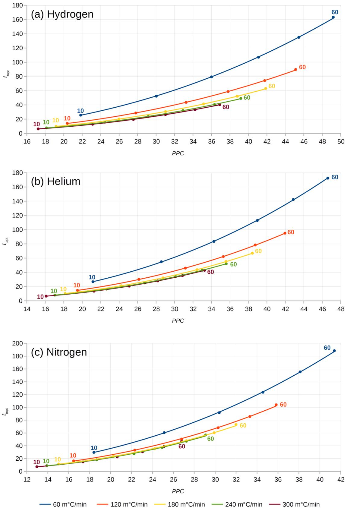
Figure 40: Different ratelengths compared for different carrier gases. Numbers on the extremes of the curves show column length in m.
