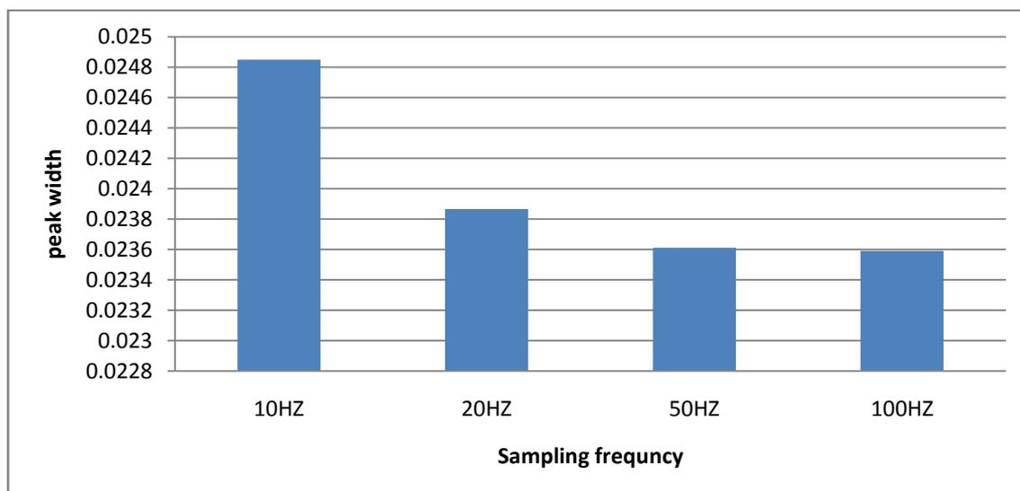
Figure 13: Peak width and detector frequency (HP-5, 10 m x 250  $\mu$ m x 0.25  $\mu$ m, 60  $^{\circ}$ C for 0 min, 30  $^{\circ}$ C/min, 30 cm/s, velocity of carrier gas, He, constant flow rate, 1:200 split ratio, 40mL/min make up gas flow rate).
