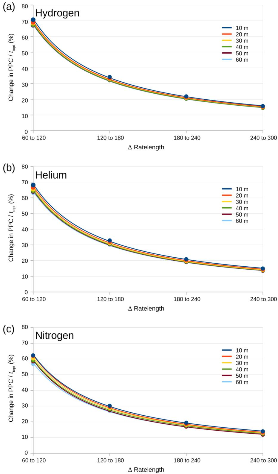
Figure 24: Percent change in  $PPC/t_{top}$  by increasing the rate length by  $60 \text{ m}^{\circ}\text{C}/\text{min}$ .
