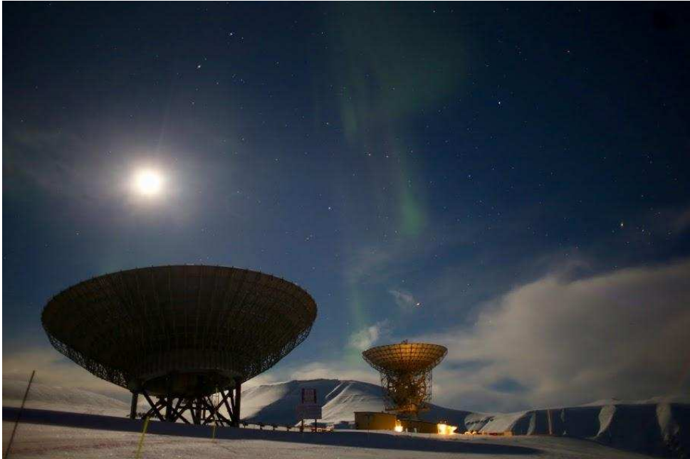
Figure 3.4: The EISCAT Svalbard Radar dishes, the fixed 42 m (left) and the steerable 32 m dish (right). Photo: Anja Strømme
