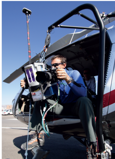
Figure 3.1.1 Photo of equipment used in acquisition of the airborne LiDAR data used in this study. This is a Riegl LMS Q240i-60 airborne LiDAR scanner including Hasselblad H1 22-megapixel camera, GNSS antenna and inertial measurement unit. The equipment is mounted on a commercial helicopter. From Rittersbacher et al. (2014a).
