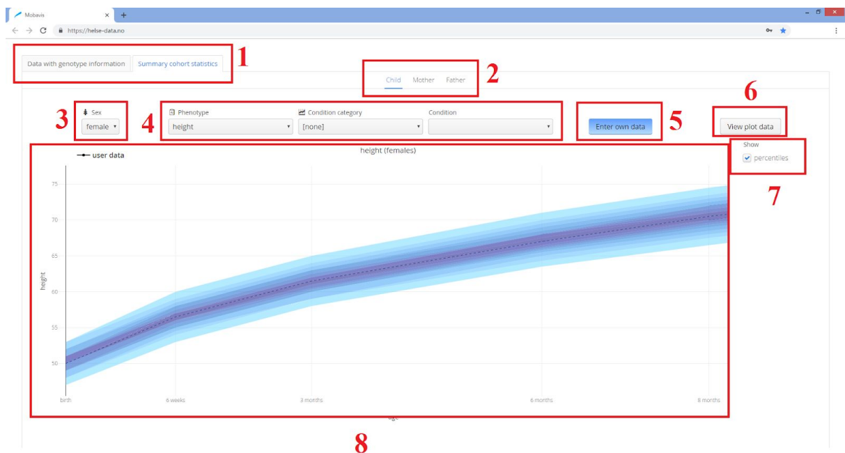
Figure 16: The appearance of the application in the web browser. The different elements of the web application visible here are: 1) the outer tabs, 2) the inner tabs for the selected outer tab, 3) a drop-down list for the selection of the sex to visualize data from (females currently selected), 4) a drop-down list for the phenotype to visualize (height currently selected), a drop-down list for the condition category (non selected) and a drop-down list for the condition, given a selected condition category (not active as no condition category selected), 5) a button that opens a pop-up letting the user enter data, 6) a button that opens
