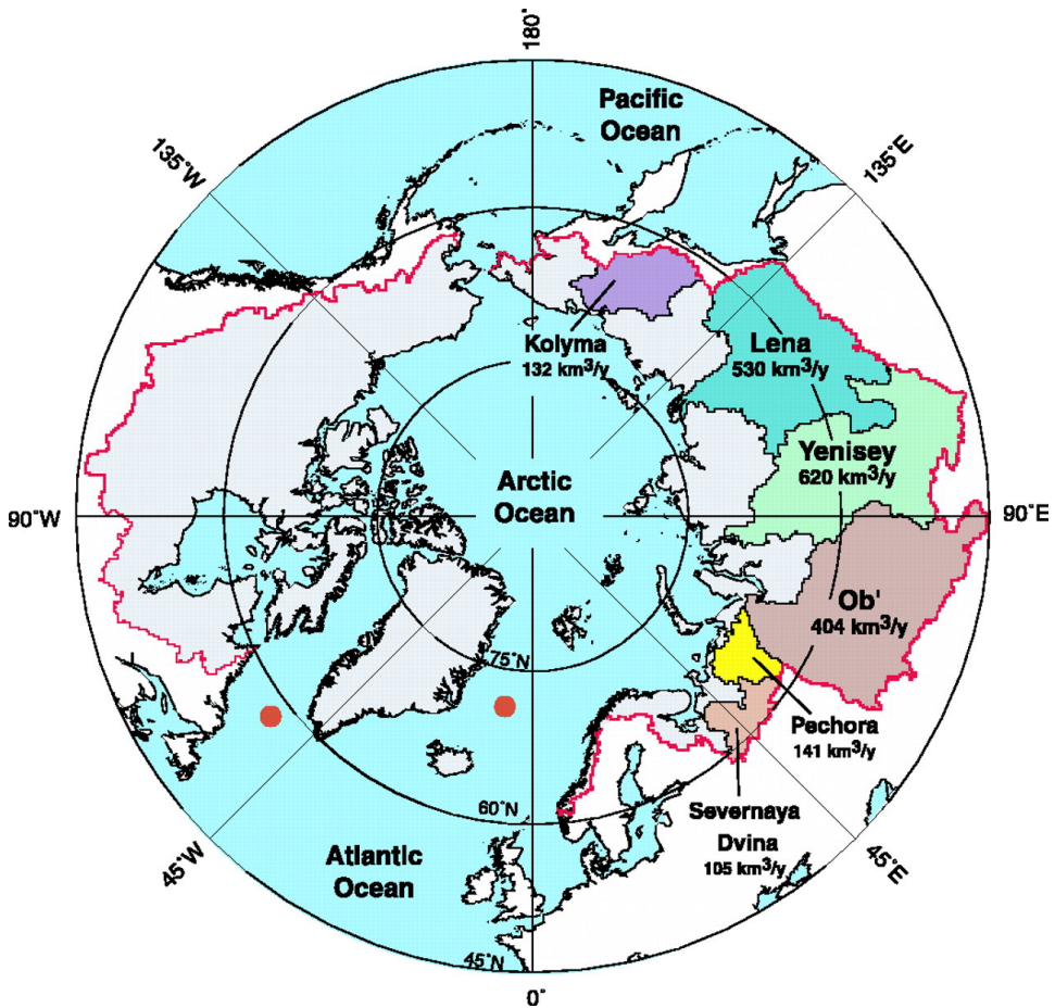
Figure 2.3: Catchment areas of river runoff to the Arctic Mediterranean. Numbers indicate freshwater fluxes from the individual rivers in \text{km}^3/\text{yr} . 1 mSv of freshwater is equivalent to 32 \text{km}^3/\text{yr} . Figure from Peterson et al. (2002).
