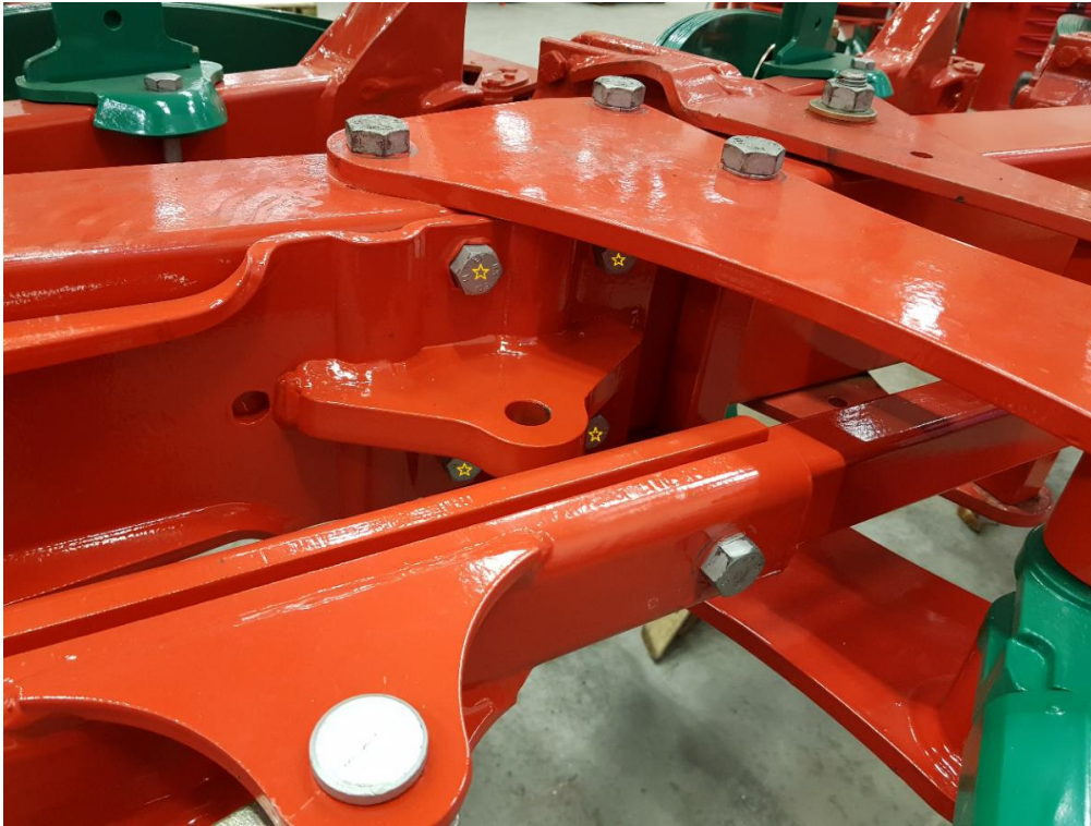
Figure 16 - Bolts rear frame support back
