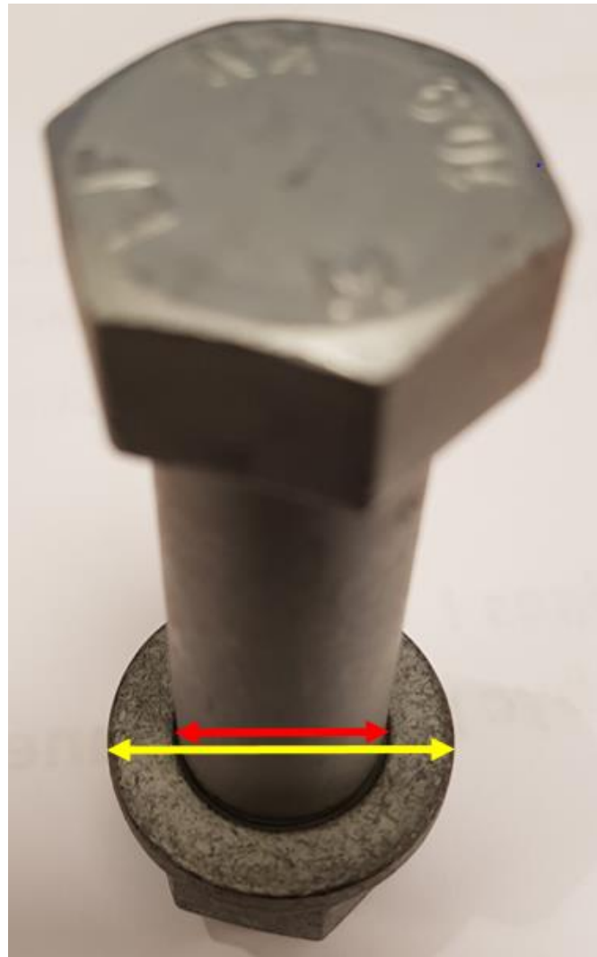
Figure 5 – Friction diameter on a KvK flange nut
