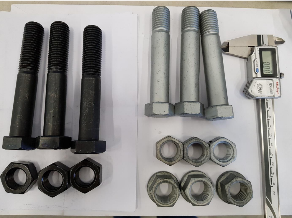
Figure 9 - Standard and KvK M20 bolts & nuts measured at KvK
