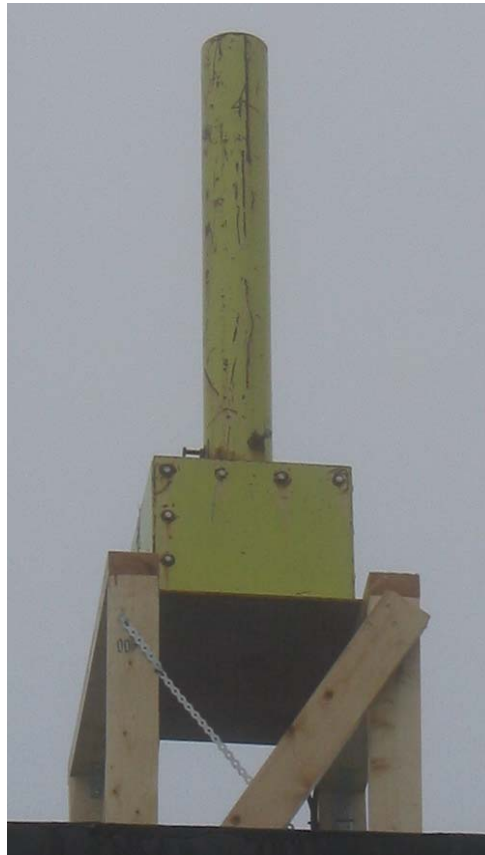
Figure 2. Ice scale mounted at Mt. Brosviksåta. The length of the cylindrical rod is 1 m and the diameter is 14 cm.
