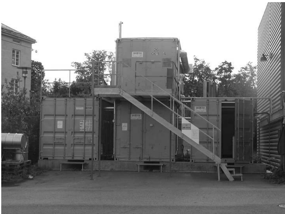
Figure 3.2 The picture shows the HP-rig. The two process containers on top of each other contain the actual rig. To the right is a technical container that carries several utility systems like the climate, power and air supply system. To the left is the gas-filling container where the fluids can be sampled, stored or filled into the process loop.
