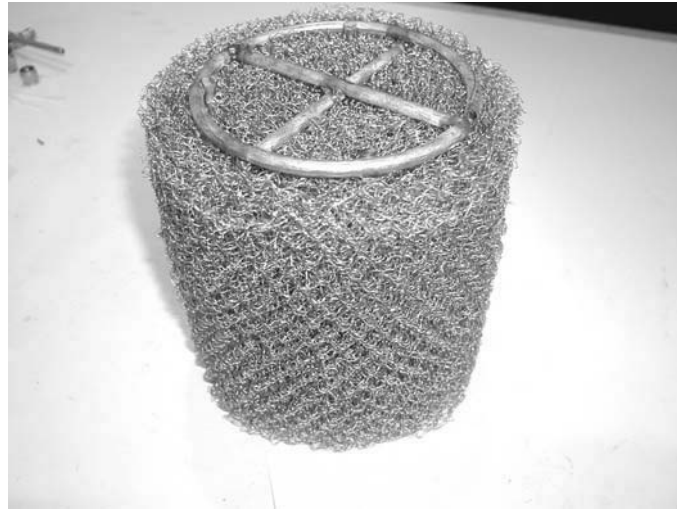
Figure 3.20 The 150 mm diameter mesh pad from Costacurta S. p. A. Vico that were used in the HP-rig.
