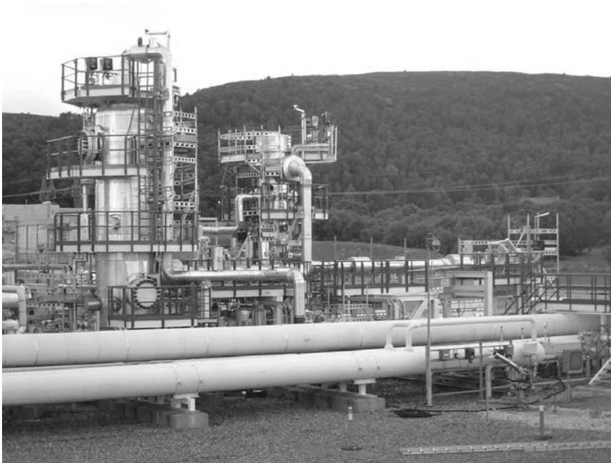
Figure 3.17 The K-lab test facility. The large scale test separator can be seen to the right. The demister scrubber is the column to the left in the picture.
