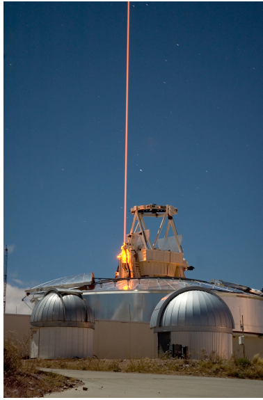
Figure 1.1: This picture is from Starfire Optical Range on Kirtland Air Force Base, New Mexico, USA (4). The laser is used to eliminate atmospheric distortions in order to get as clear images as possible of objects in space.
