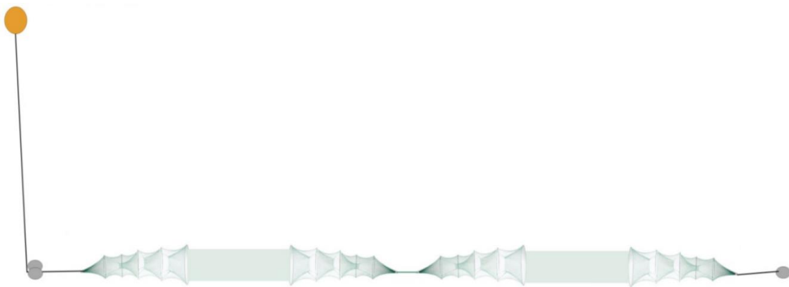
Figure 2.3.3 – One fyke net setting, consisting of two doubled fyke nets, where each has a 6 m lead net in the middle and two cod ends. In total 4 cod ends (van der Meeren 2017).
