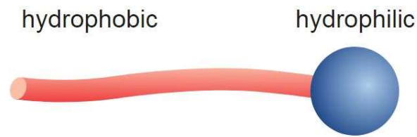
Figure 3.1: Schematic structure of a surfactant [34].
