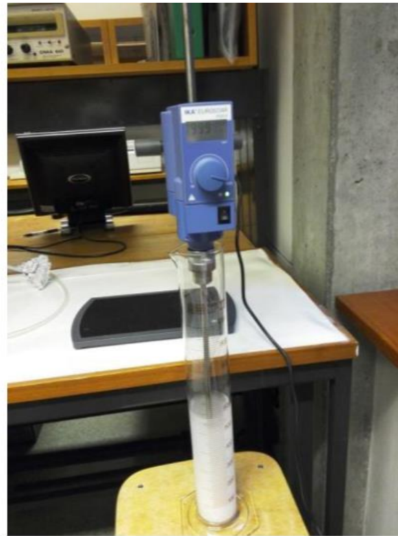
Figure 29: On the left a schematic of foam stability test modified from (Schramm, 2006, and on the right example of foam preparation.
