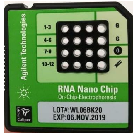
Figure 5. RNA chip. Well 1-12 in column 1-3 are used for samples and the 4 th column is used for gel-dye mix and ladder.
