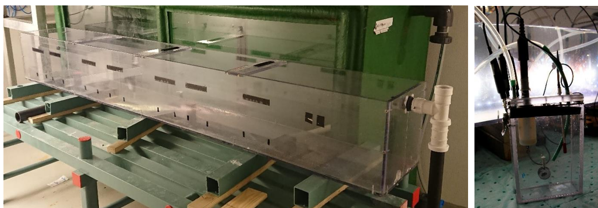
Figure 5 The big tank (left) where the six small incubation chambers were placed (right). The incubation chamber here showed with its lid and the connected probes and pipes.
