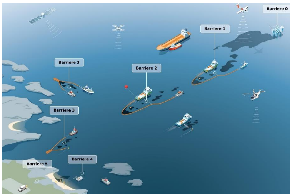
Figure 1. Oil spill response strategies according to barrier; 1, close to the source; 2, between the source and the coast; 3, near the coast; 4, along the coastline; 5, at shore (Courtesy of NOFO).
