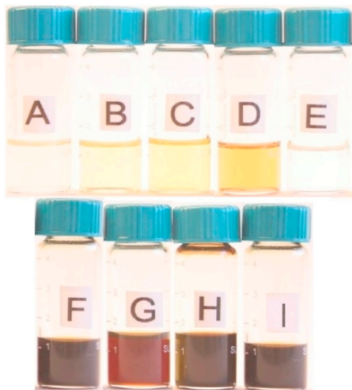
Fig. 1. Visual presentation of the oils included in the study. The condensates (A–E) were clear or yellow and the light crude oils (F–I) were dark red or brown. (For interpretation of the references to color in this figure legend, the reader is referred to the web version of this article.)
