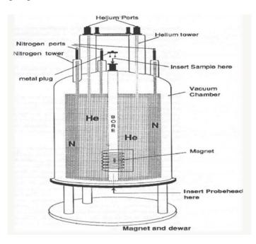
Figure 6: The inside of a modern cryomagnet[13]
