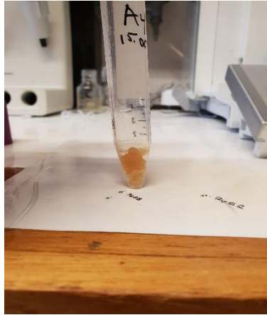
Figure 4.3.4: Lyophilized chitosan hydrogel after one week of incubation in water.
