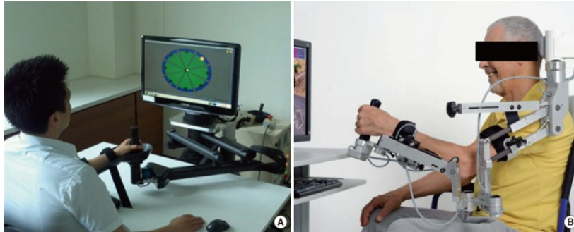
Fig. 1.1 Example of robotic devices for motor functions training, distributed under the terms of the Create Commons Attribution Non-Commercial Licence (Chang and Kim, 2013).
