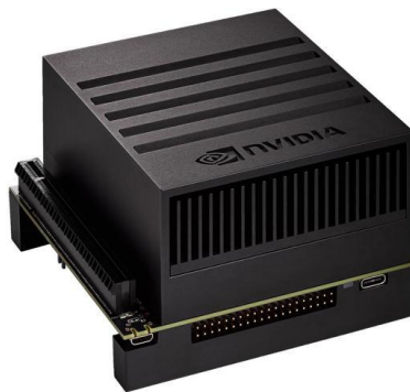
Fig. 6.8 NVIDIA’s Jetson Xavier, the computing device used on the robot in our system. Image from NVIDIA’s homepage ( NVIDIA, 2018 ).
